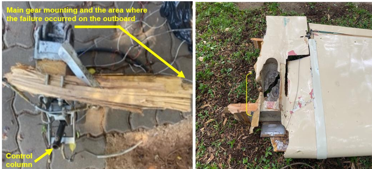
Figures 9/10: The outboard gear mount area showing where the failure occurred (left picture). The right wing and the right gear wheel well/fairing after they were reconstructed post-accident (right picture).
