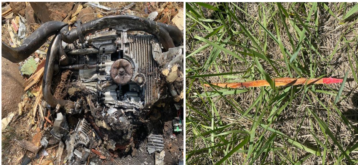
Figures 11/12: The fragmented VW 2180 CC engine (left picture). Wooden blade remnant indicates an engine that was operating prior to impact (right picture).
