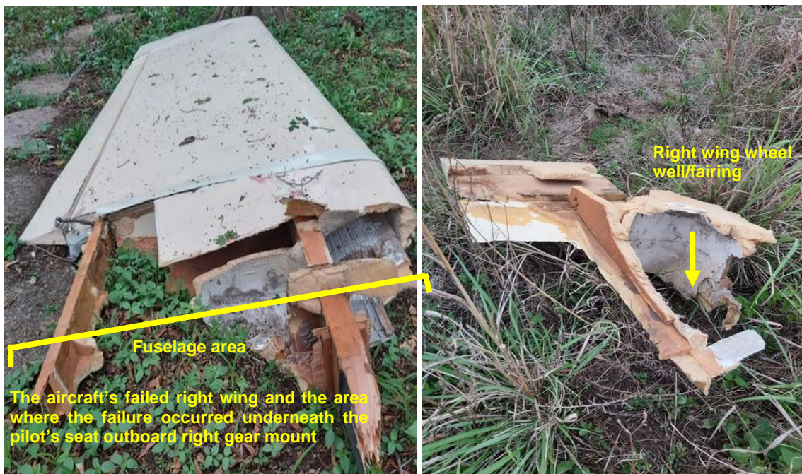
Figures 7/8: The right wing was found in an inverted position (left picture). The right gear wheel well/fairing at the accident site (right picture).
