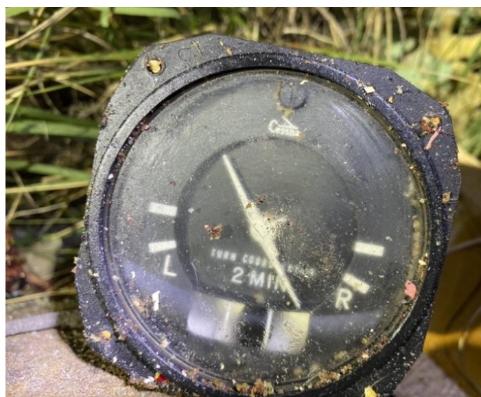
Figure 5: The turn and bank co-ordinator indicator showing the attitude of the aircraft prior to impact.
