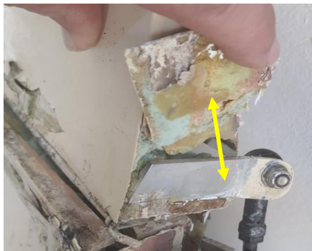
Figure 17: The aileron and bell crank separation caused by flutter.
