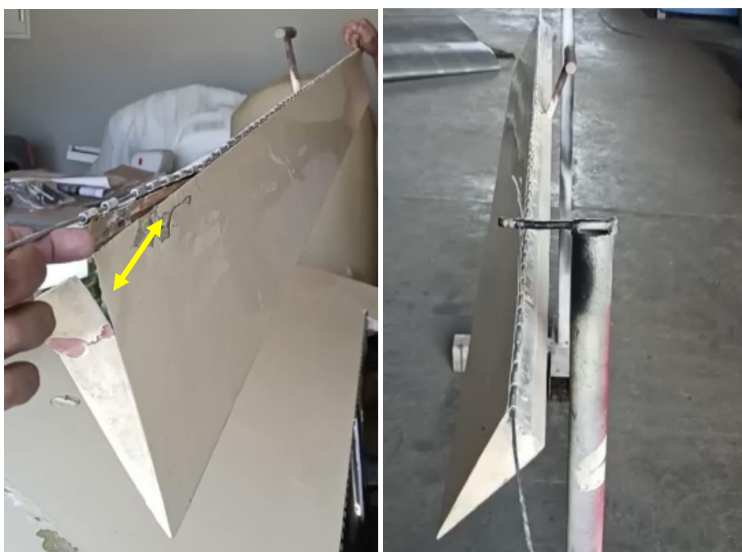
Figures 13/14: The aileron after it was removed from the failed right-wing (left picture). The aileron after it was glued together (right picture).
