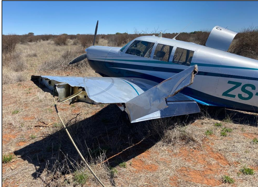
Figure 1: ZS-FRO's damaged left wing. (Source: Pilot)
