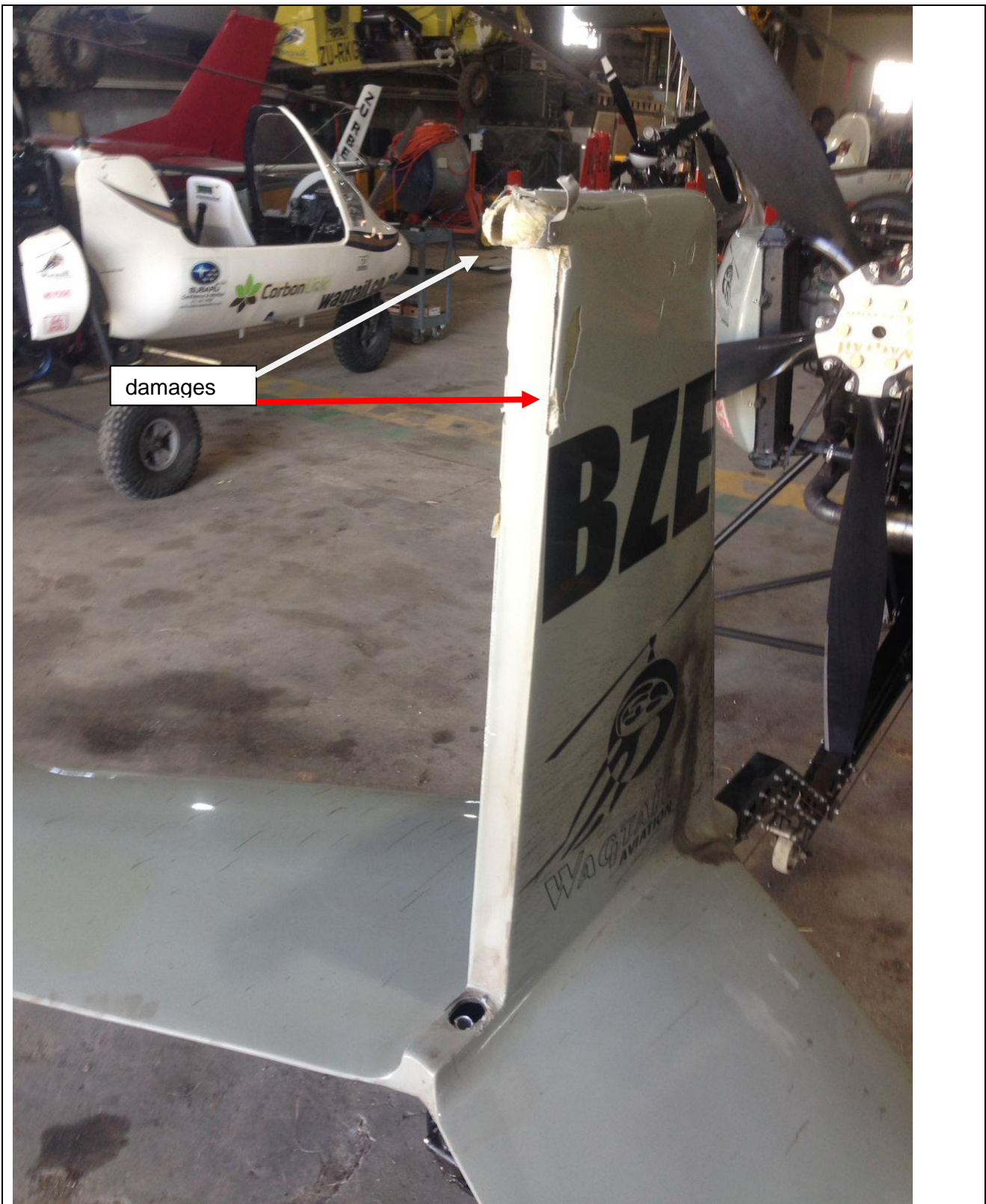
Figure 1: Damage on the rudder. (Source: Pilot)
