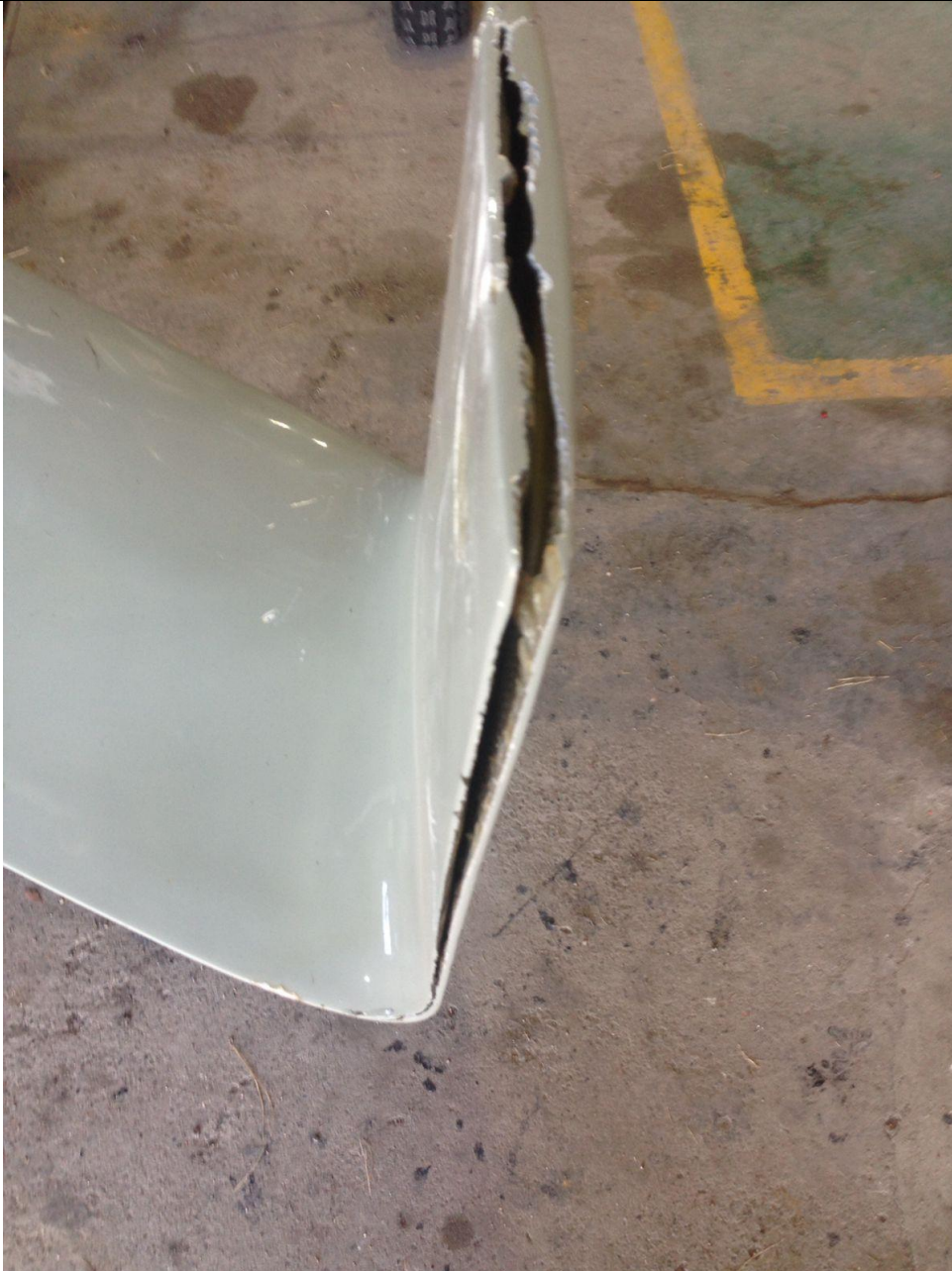
Figure 2: Damaged winglet. (Source: Pilot)
