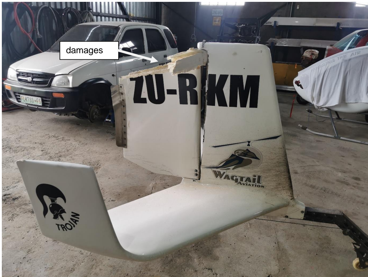
Figure 1: Damage on the rudder. (Source: Pilot)
