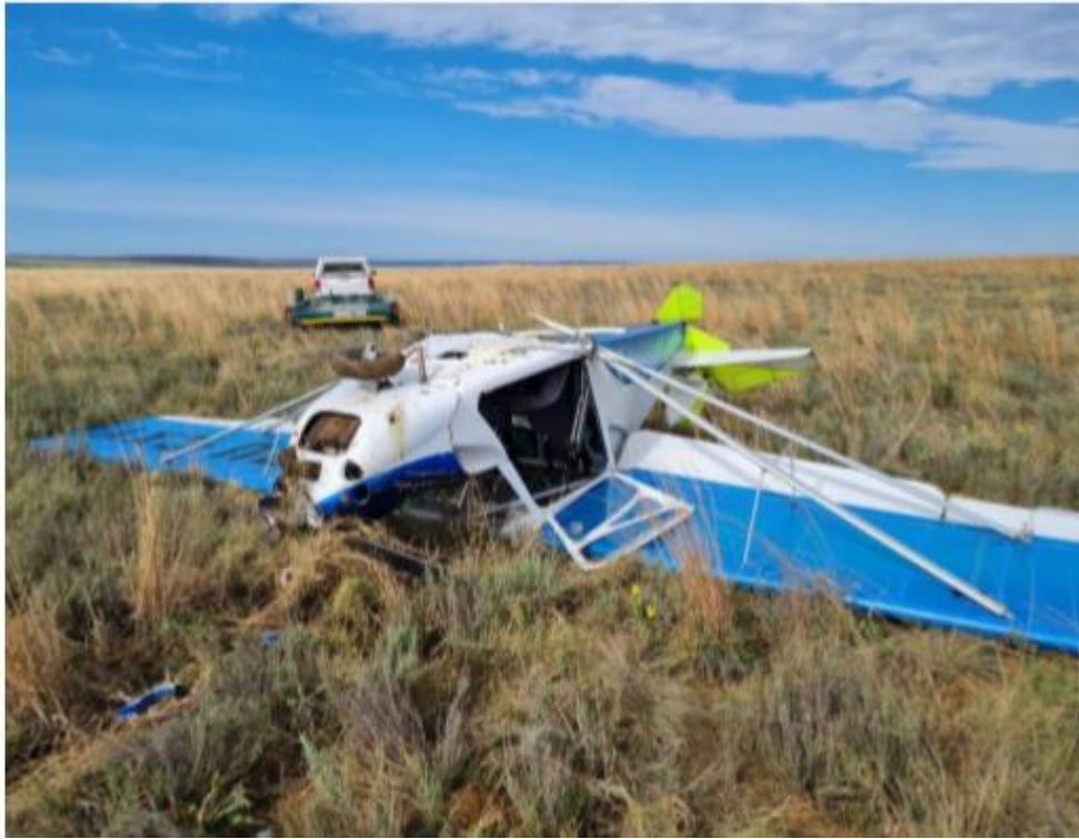
Figure 3: The aircraft as it came to rest in an inverted position. (Source: Operator)
