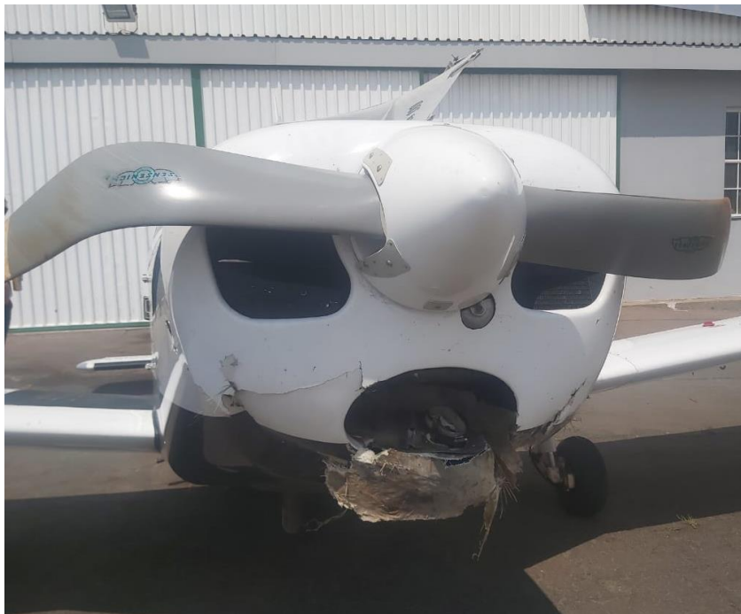
Figure 2: Close-up view of damages on the lower cowling and propellers.
