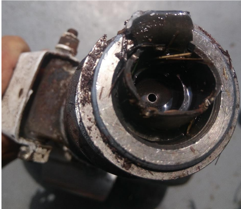
Figure 3: Close-up view of the damaged nose gear steering tube assembly.
