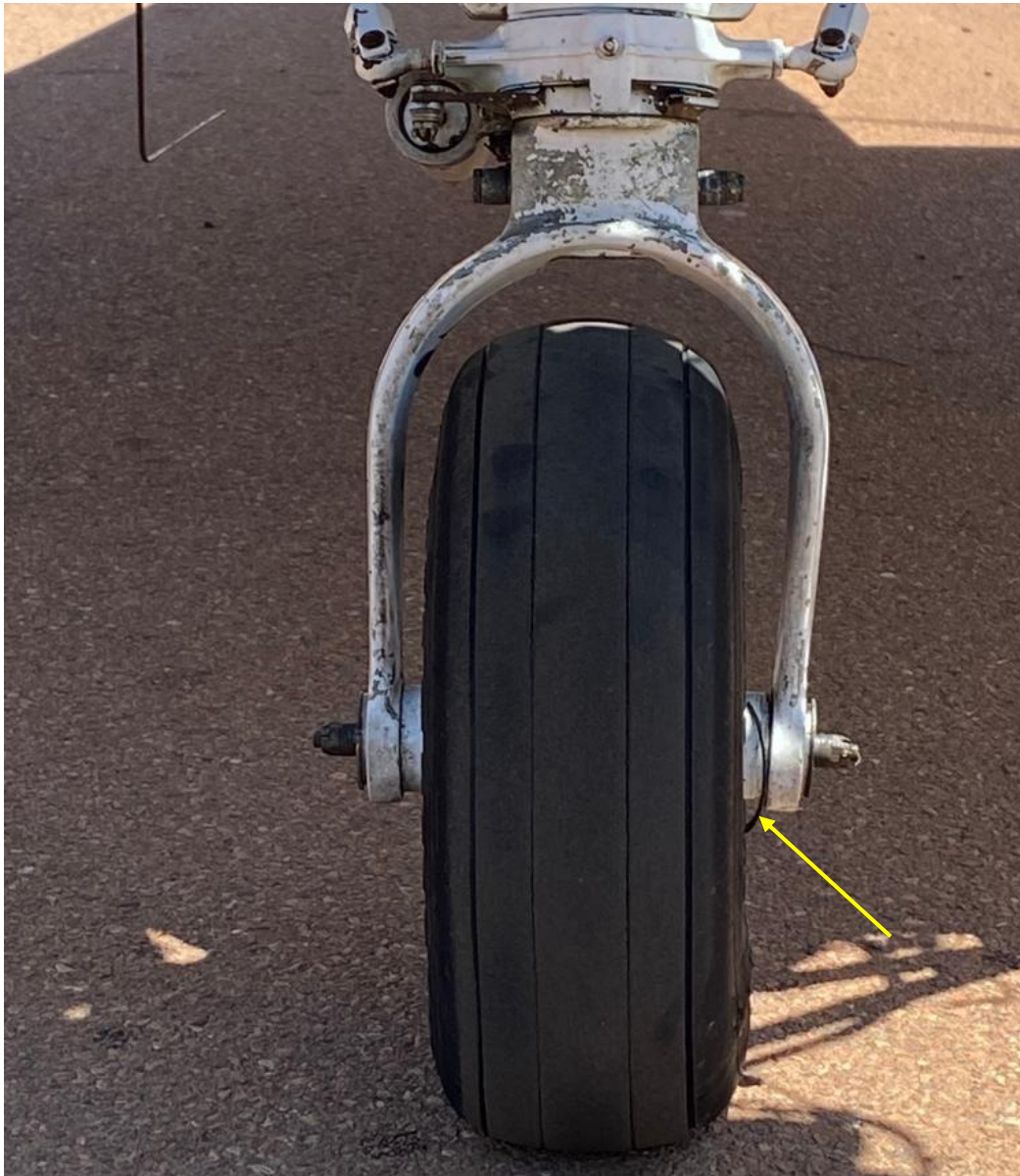
Figure 1: The nose gear fork displays slight bending deformation and damage at the axle.
