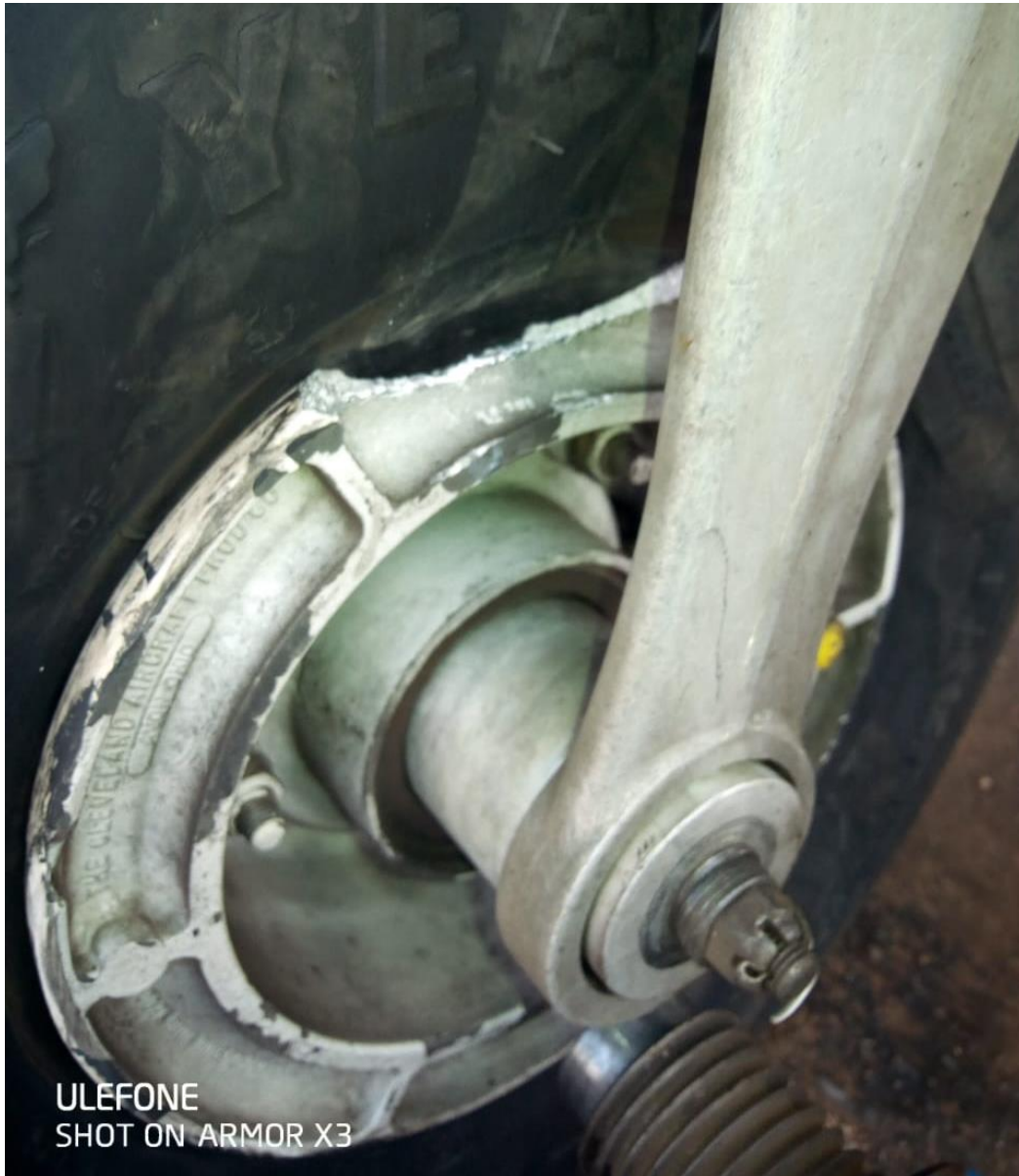
Figure 1: The nose wheel rim sustained damage during hard landing.
