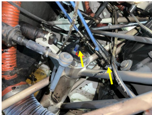
Figure 1: Some melted wiring post-accident. (Source: Operator).
