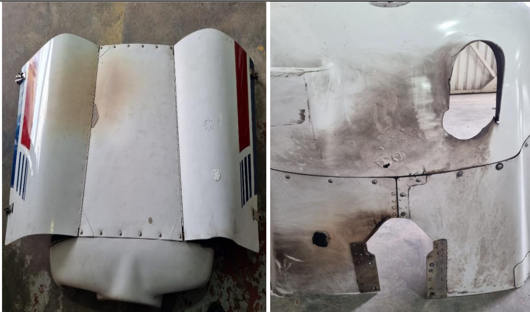
Figures 2/3: Fire damage at the top and bottom cowlings. (Source: Operator).
