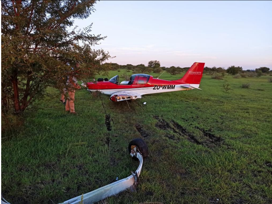
Figure 1: The aircraft at the accident site and the main landing gear strut in the foreground. (Source: Pilot)
