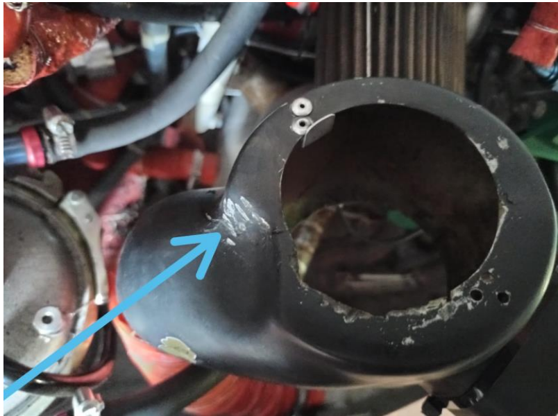
Figure 4: Witness marks left on the air-filter housing.
