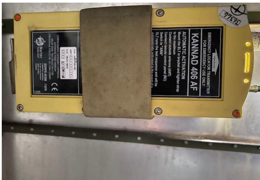
Figure 13: The ELT installed on the aircraft's tail-section.
