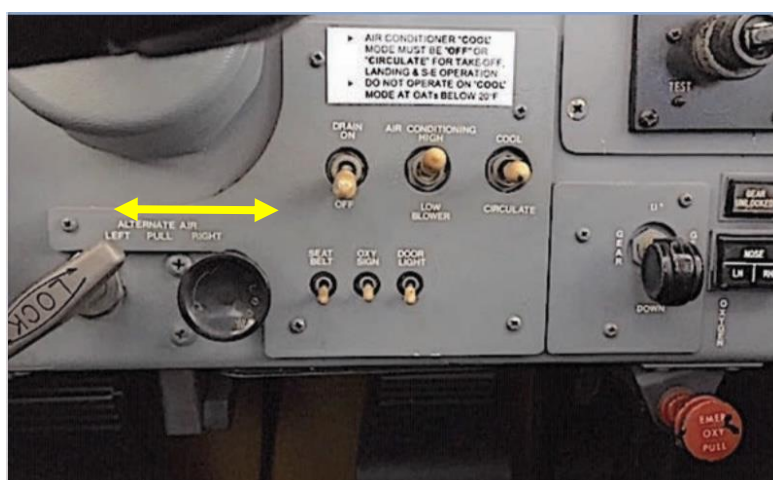
Figure 9: The left and right ALTERNATE AIR levers in a closed (OFF) position.
