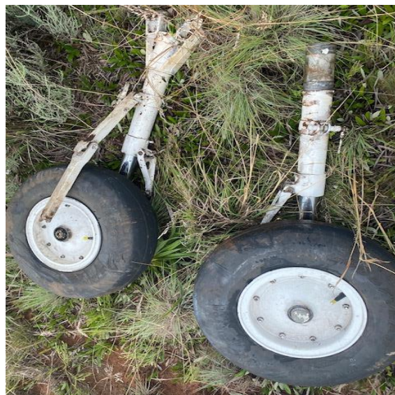
Figure 7: View of the broken main landing gear struts with the wheel assemblies still attached.
