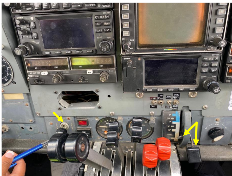
Figure 8: A view of the aircraft's console showing the landing gear selector handle in an extended position and the flap position indicator at 45°.
