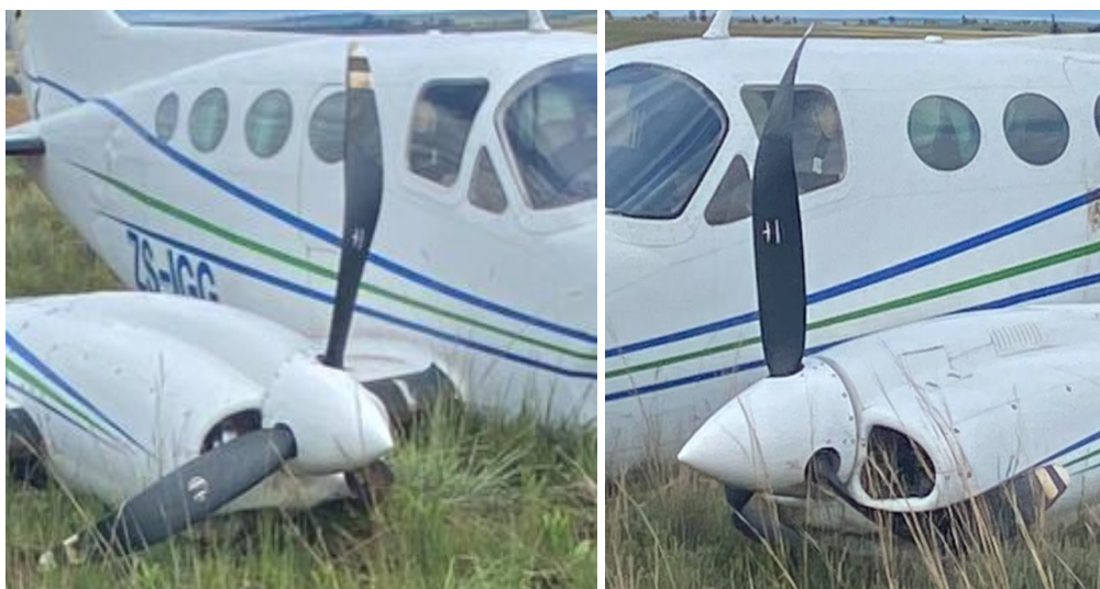
Figures 11 and 12: Pictures showing neither of the propellers feathered.
