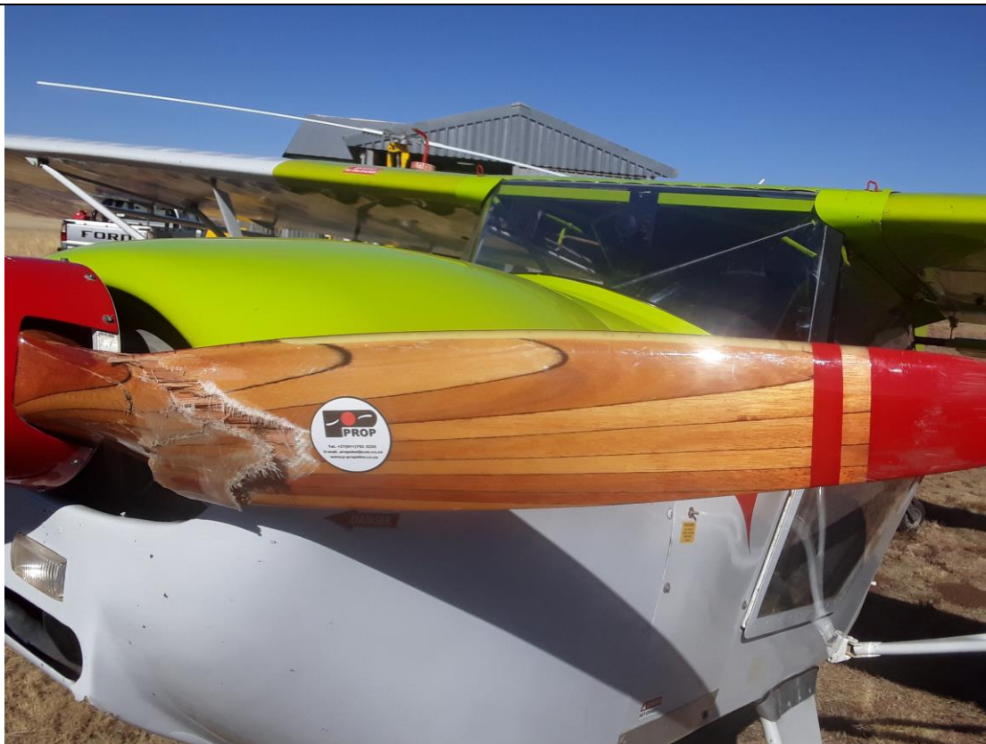
Figure 1: The damaged propeller. (Source: Pilot)
