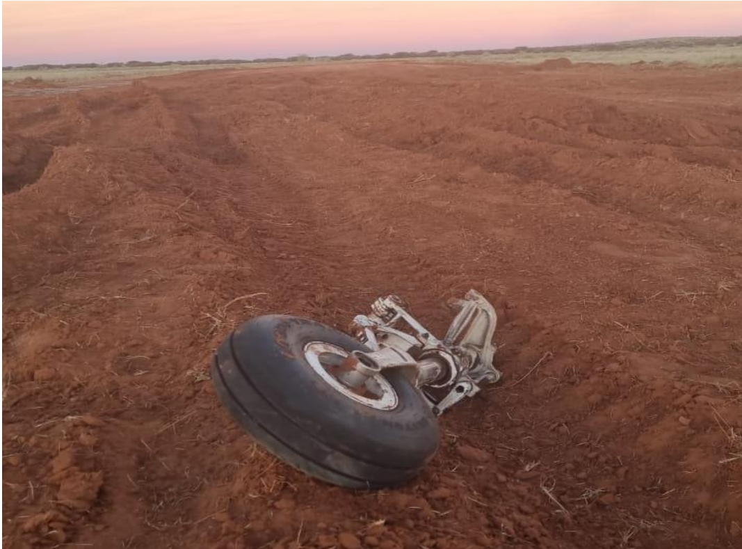
Figure 1: Heap of sand on RWY28 and the detached nose gear assembly. (Source: EMS)
