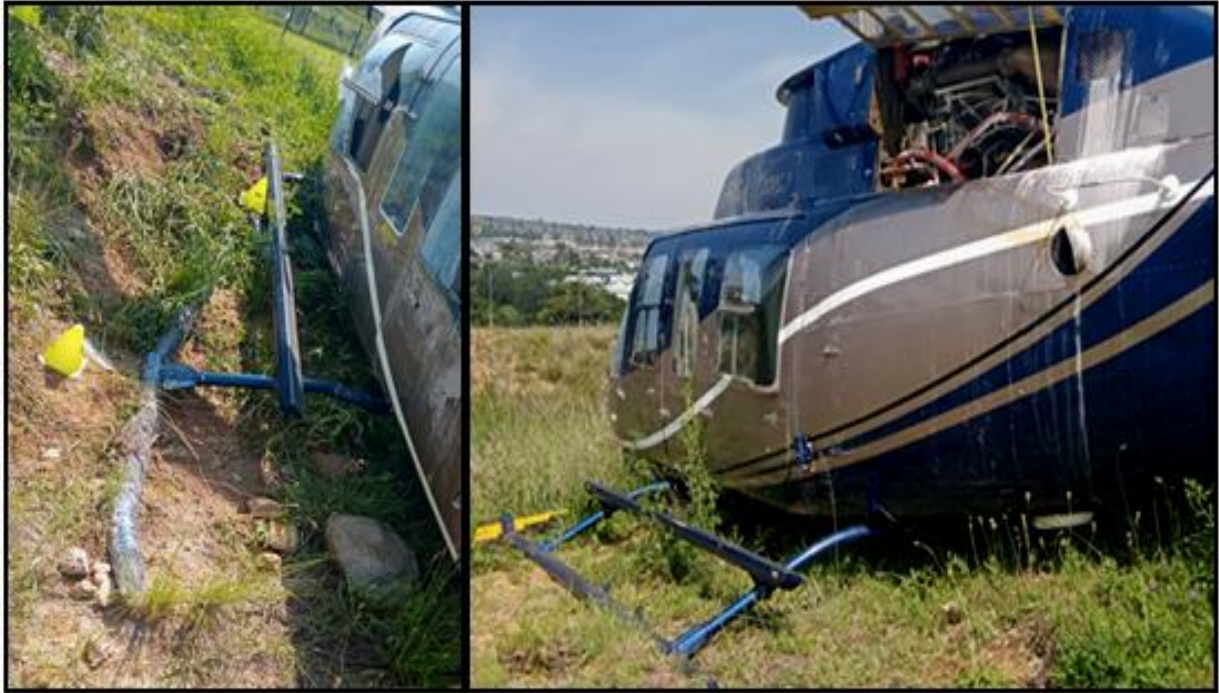
Figure 4: The right- and left-side skid gear damages sustained during the accident
