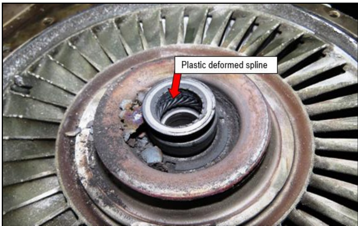
Figure 13: Shows the plastic deformation of the splined coupling due to overheating the turbine section (Source: Manufacture Report)
