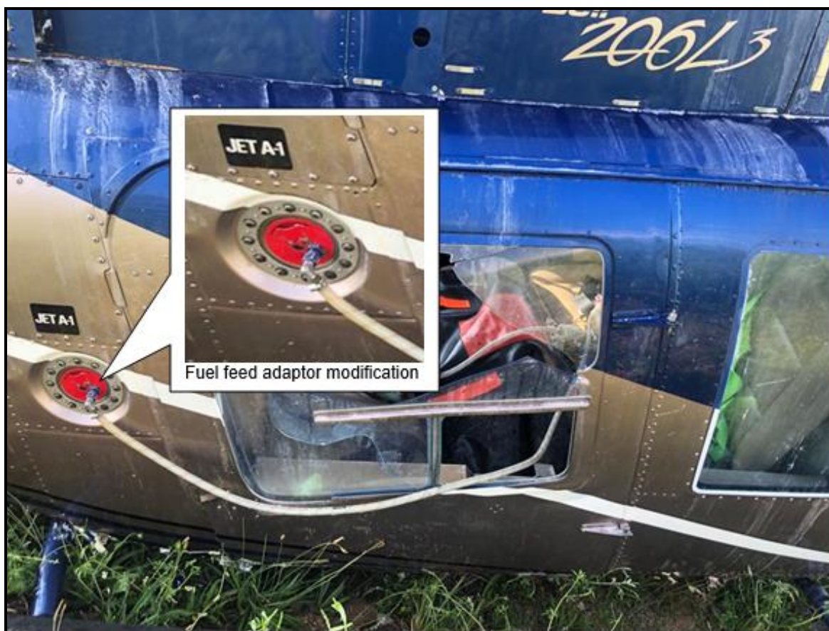
Figure 9: The fuel feeder line connected to the right-side fuel tank cap with a connecting adaptor.
