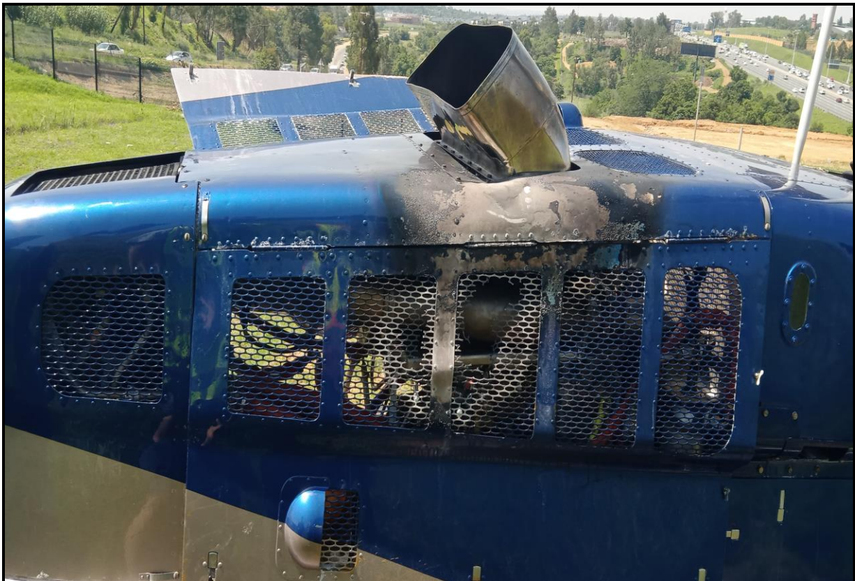
Figure 5: Heat damage on the right-side engine cowling.
