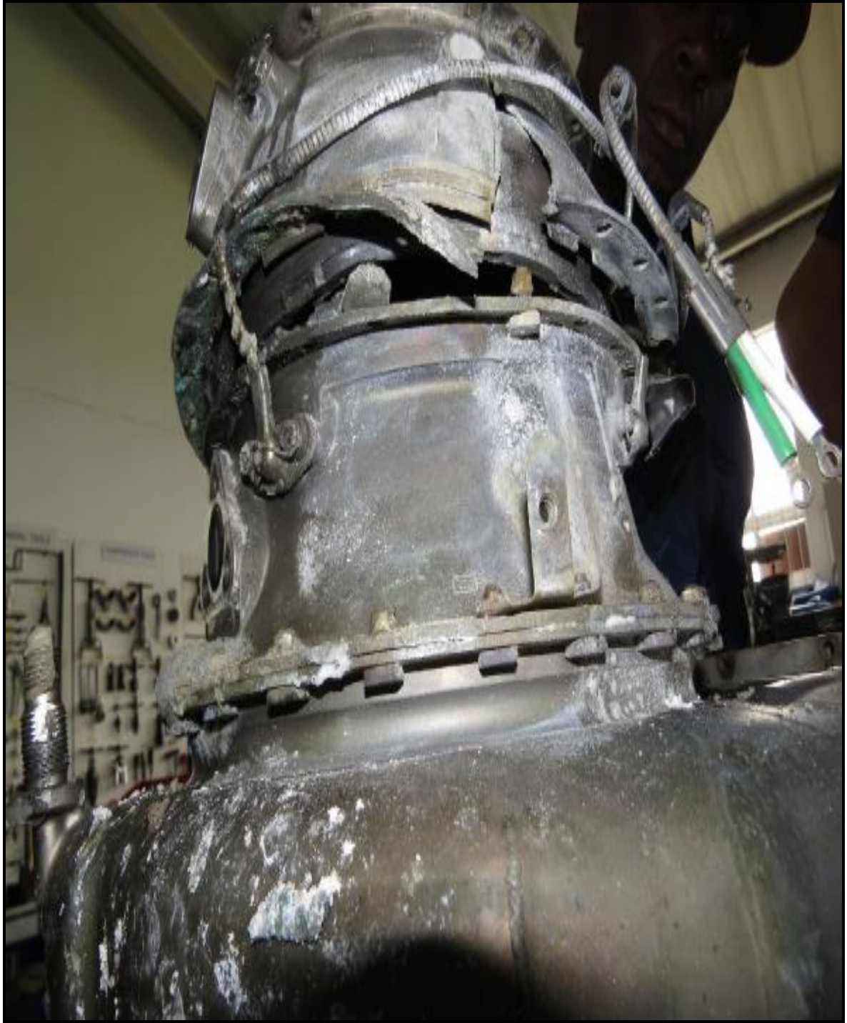
Figure 11: Turbine section damages.
