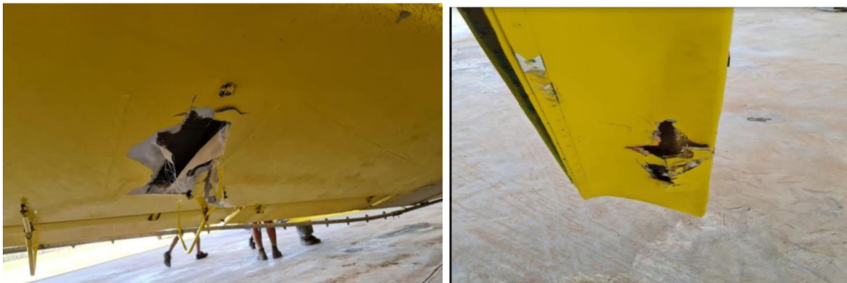
Figure 2 and 3: Damage on the left wing (left picture); damage on the right wing (right picture). (Source: Operator)
