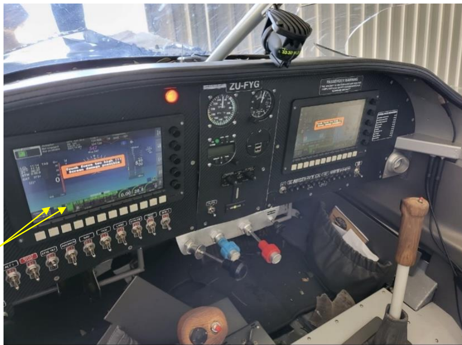
Figure 4: The cockpit showing the EFIS glass panels and fuel level display.
