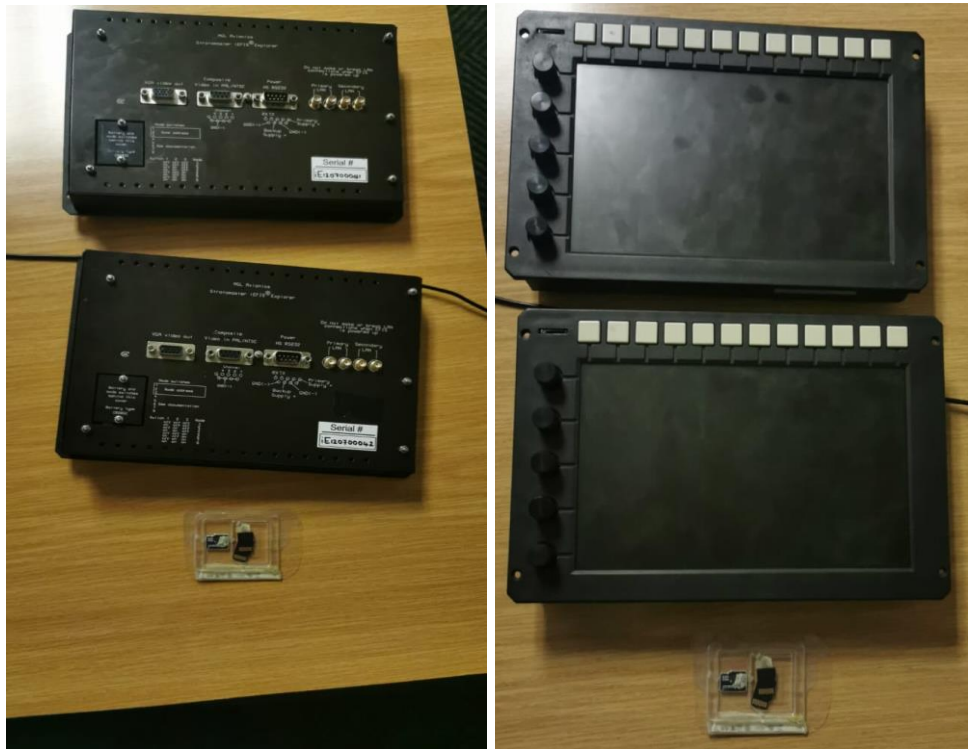
Figures 9 and 10: The EFIS glass panels with SD cards.
