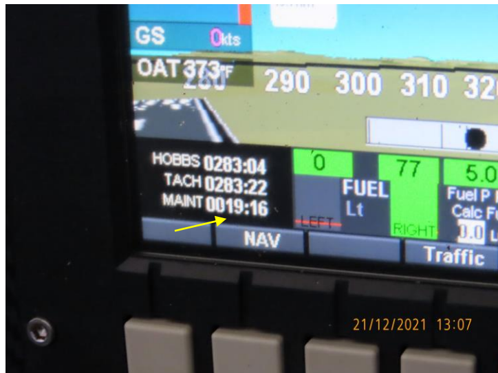
Figure 11: The left-side EFIS glass panel showing fuel indications, fuel pressure at 5.0 bar, and 19 minutes flight time.
