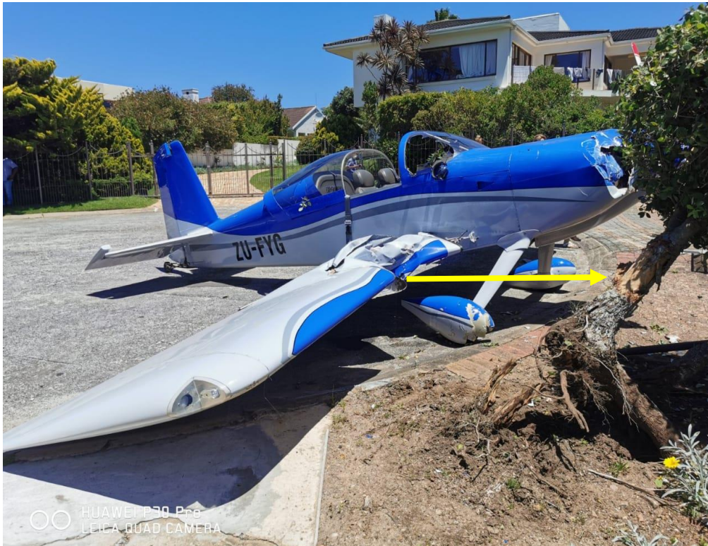
Figure 2: Damage to the right wing after it uprooted a tree. (Source: Fire Chief)
