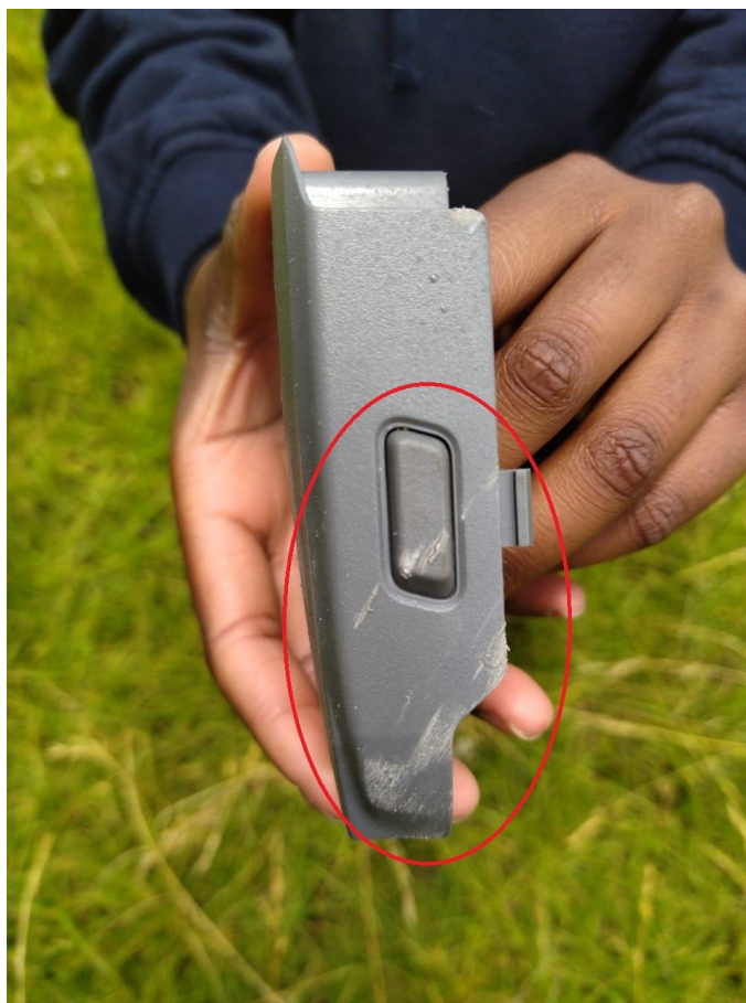
Figure 3: Battery cover that was recovered with scuff marks. (Source: Pilot)
