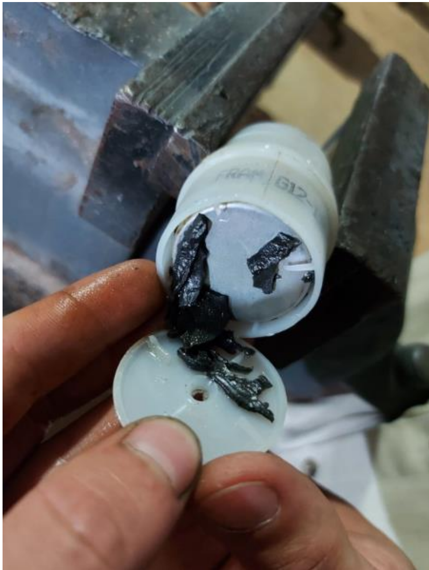
Figure 2: A clogged fuel filter. (Source: AMO)
