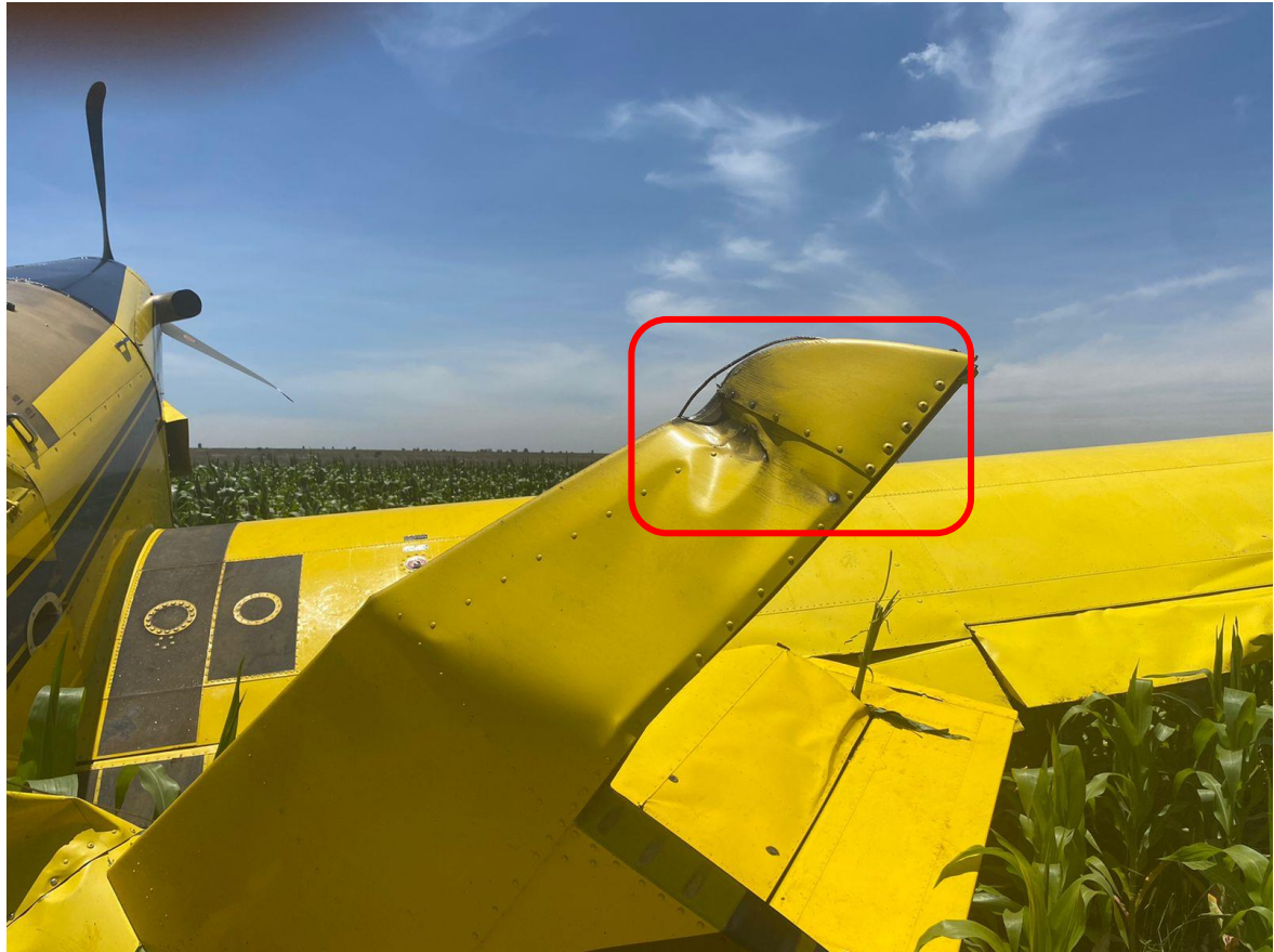
Figure 1: The area on the vertical stabiliser where it impacted the electrical cables.
