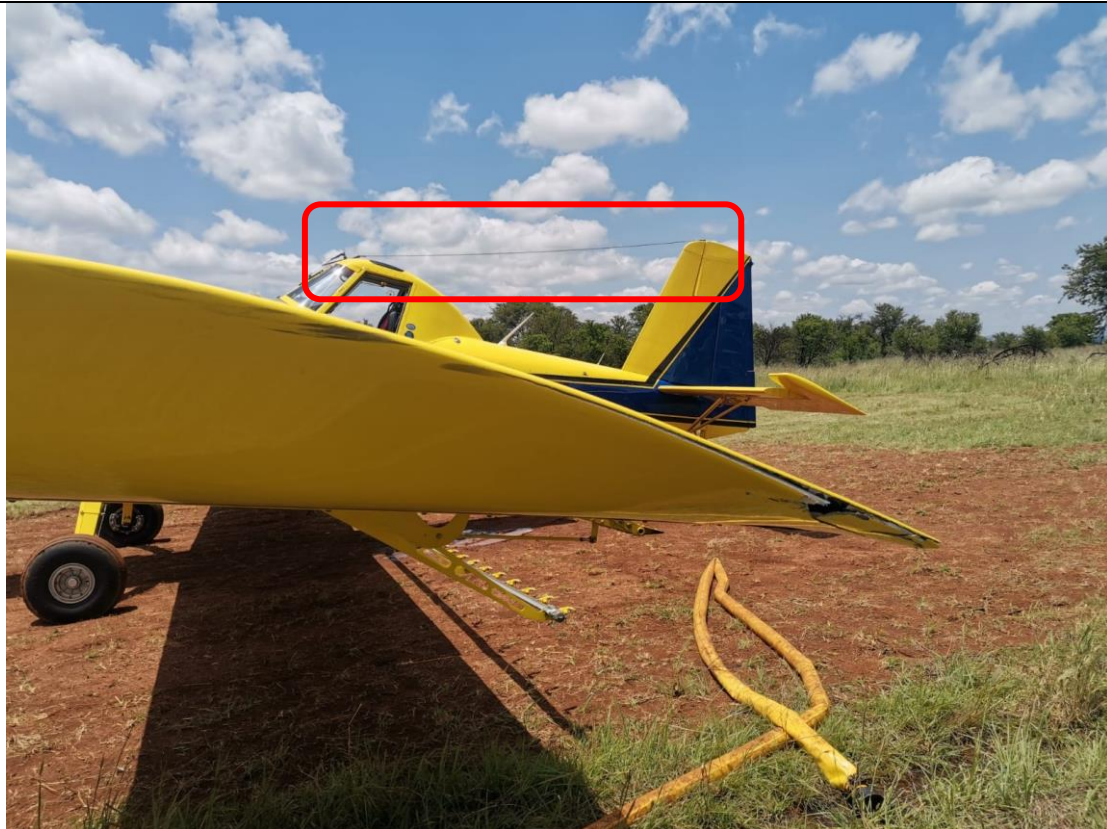
Figure 4: A similar type of aircraft with the cable deflector in the red window.
