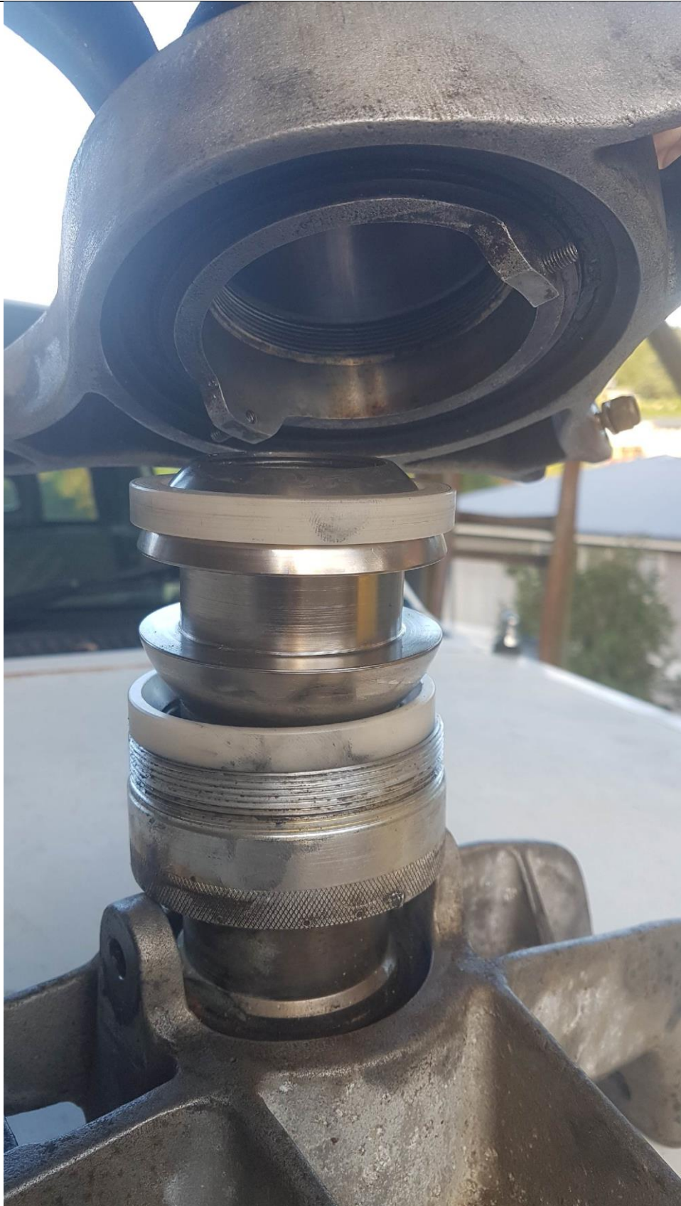
Figure 6: The slider ball adjustment collar assembly with the rotating swashplate at the top. (Source: Helicopter pilot/owner)
