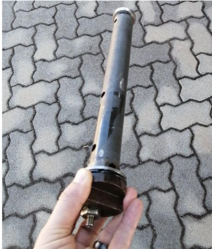
Figure 1: Damage to the nose gear oleo stop bolt. (Source: Operator)
