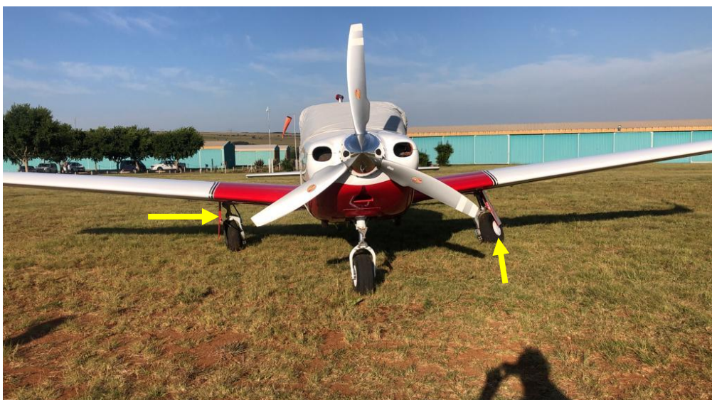
Figure 2: The aircraft with the bent main landing gear.
