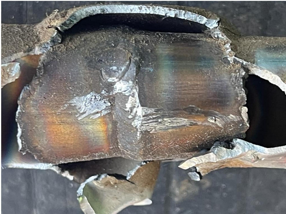
Figure 4: The damage on the nose wheel gear fork. (Source: Owner)
