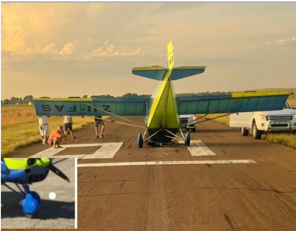
Figure 1: The aircraft's nose wheel fork broke off just before the take-off roll. Inset: The wheel spat/fairing. (Source: Pilot)
