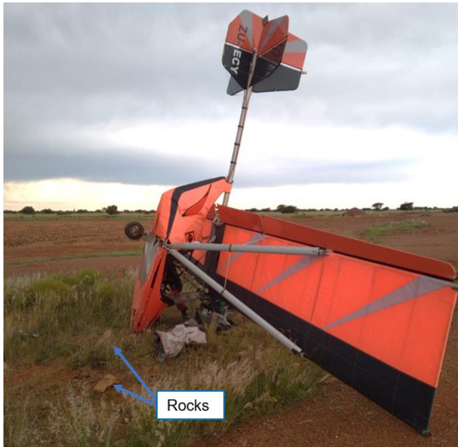
Figure 1: The aircraft as it came to rest after colliding with a rock. (Source: Owner)
