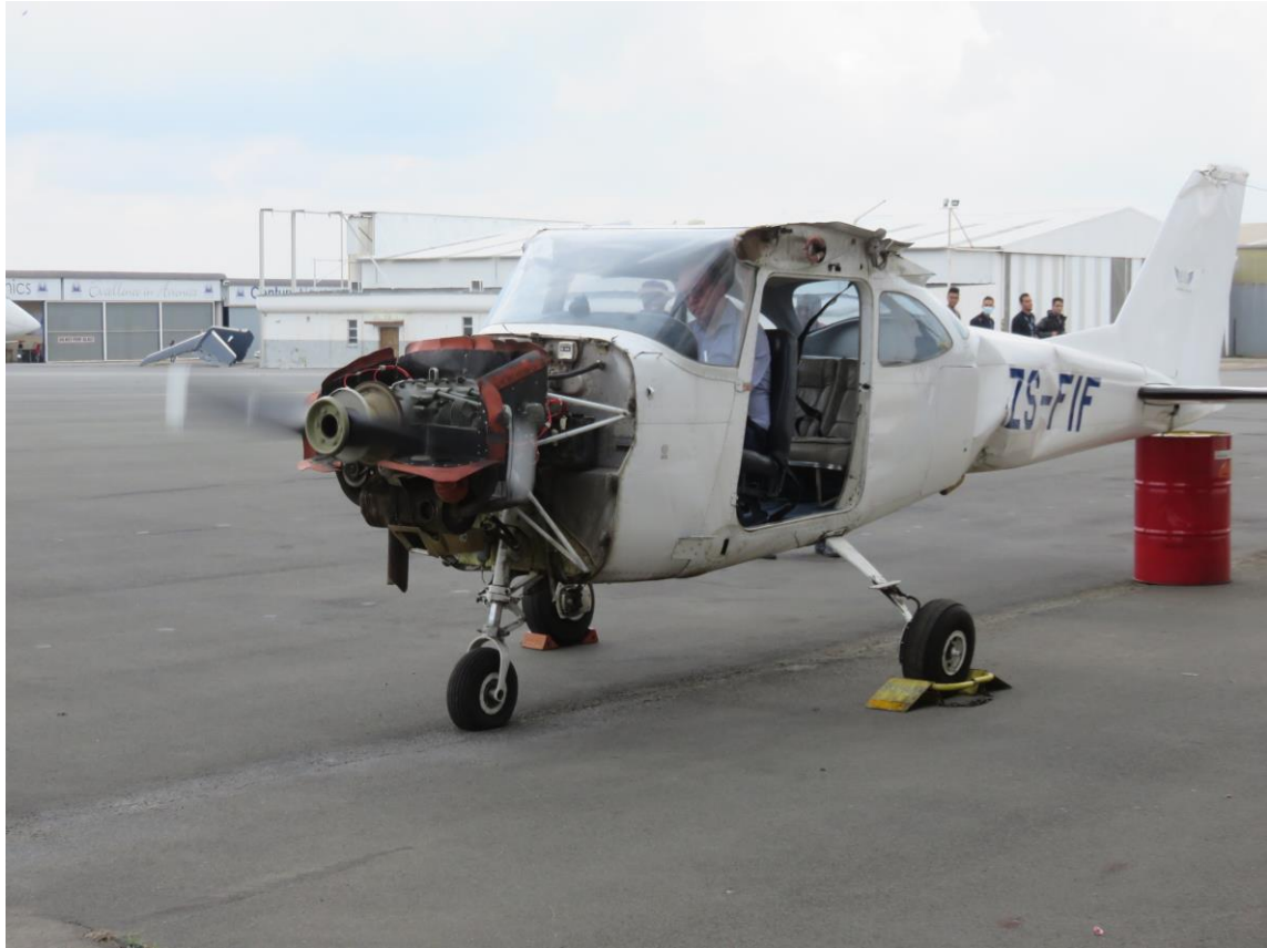
Figure 7: An engine ground run was performed, and the engine ran without a problem.
