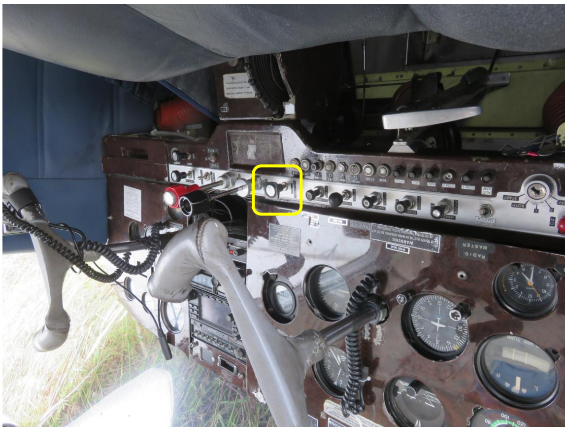
Figure 8: The position of the carburettor heat lever (in the yellow window) taken on-site.
