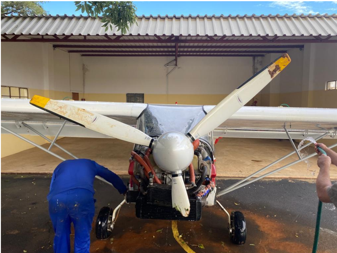
Figure 3: Damage to the propeller and engine bay. (Source: Pilot)
