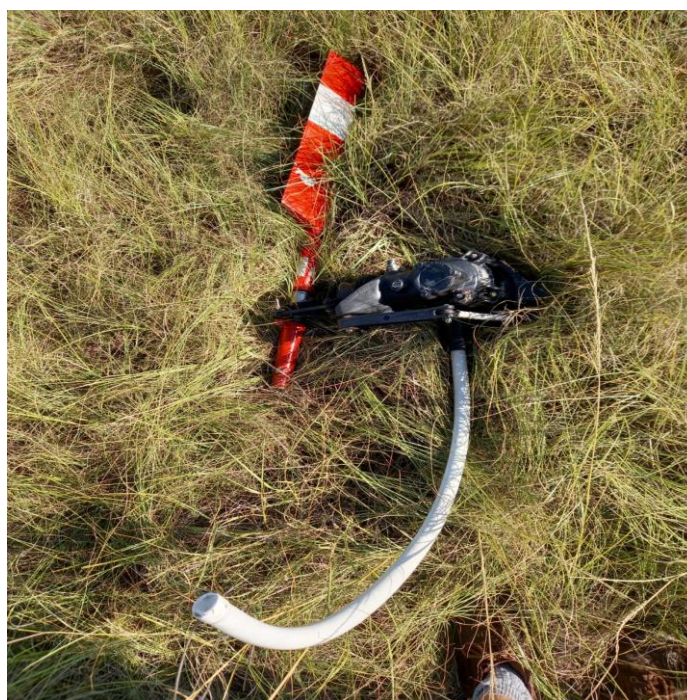
Figure 2: The tail rotor and gearbox with one blade missing. (Source: Operator)
