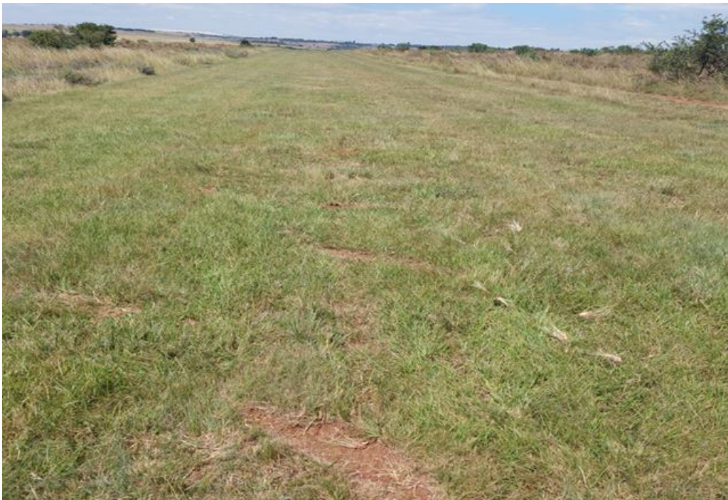
Figure 5: Propeller marks on the ground.
