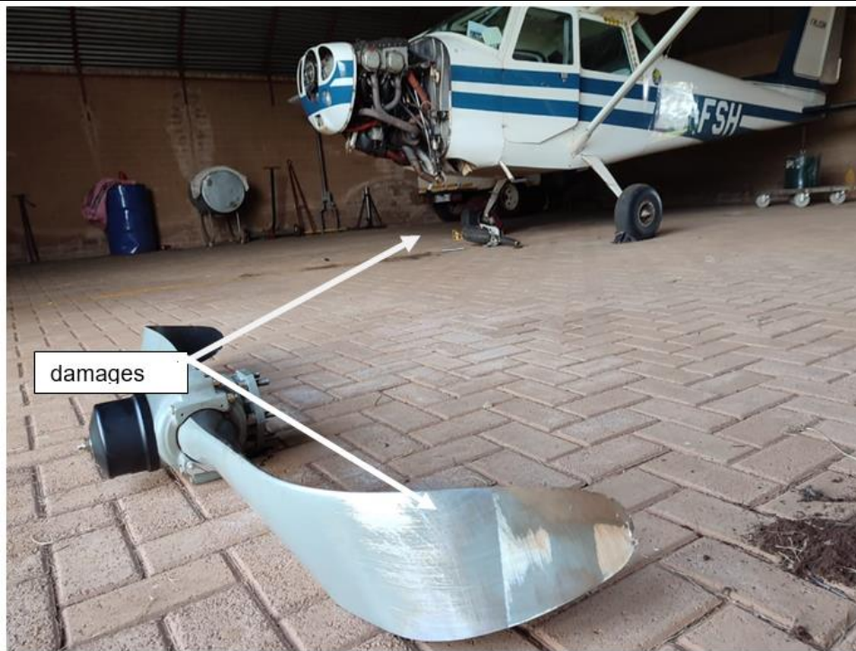
Figure 1: The damaged propeller and nose landing gear.
