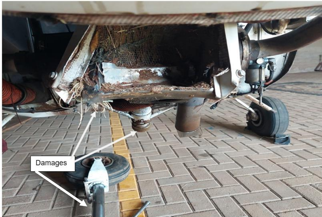
Figure 2: Damage on the nose landing gear.
