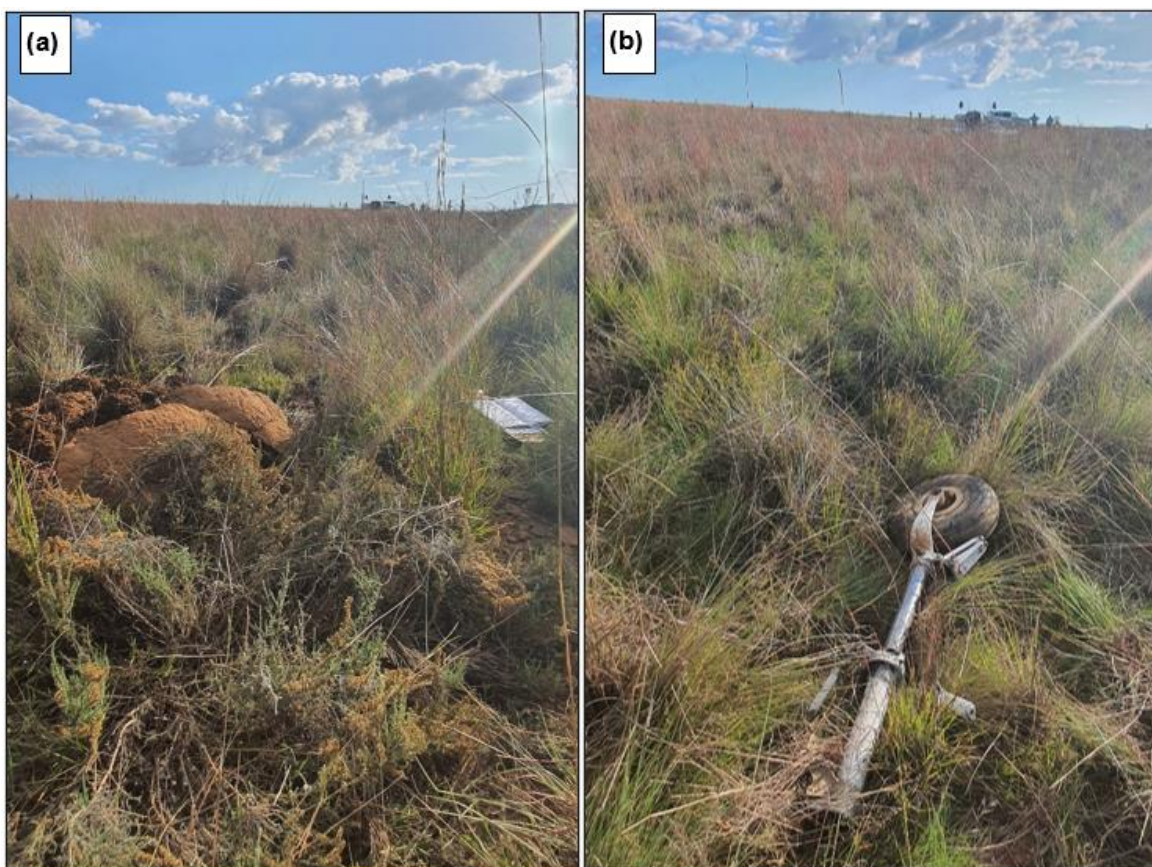
Figure 2: (a) The anthill with which the nose gear collided. (b) Location of the nose landing gear strut in relation to the main wreckage.
