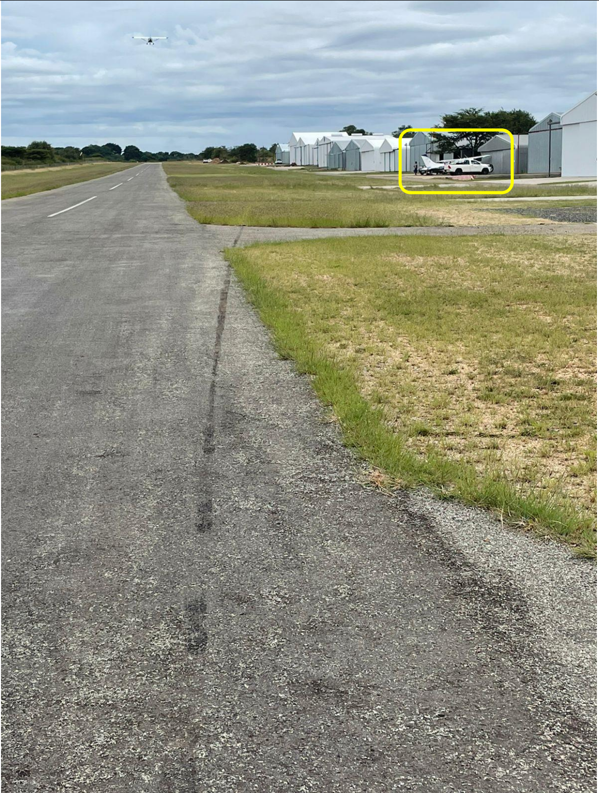
Figure 2: Tyre markings of the right main wheel and the accident aircraft in the yellow window.
