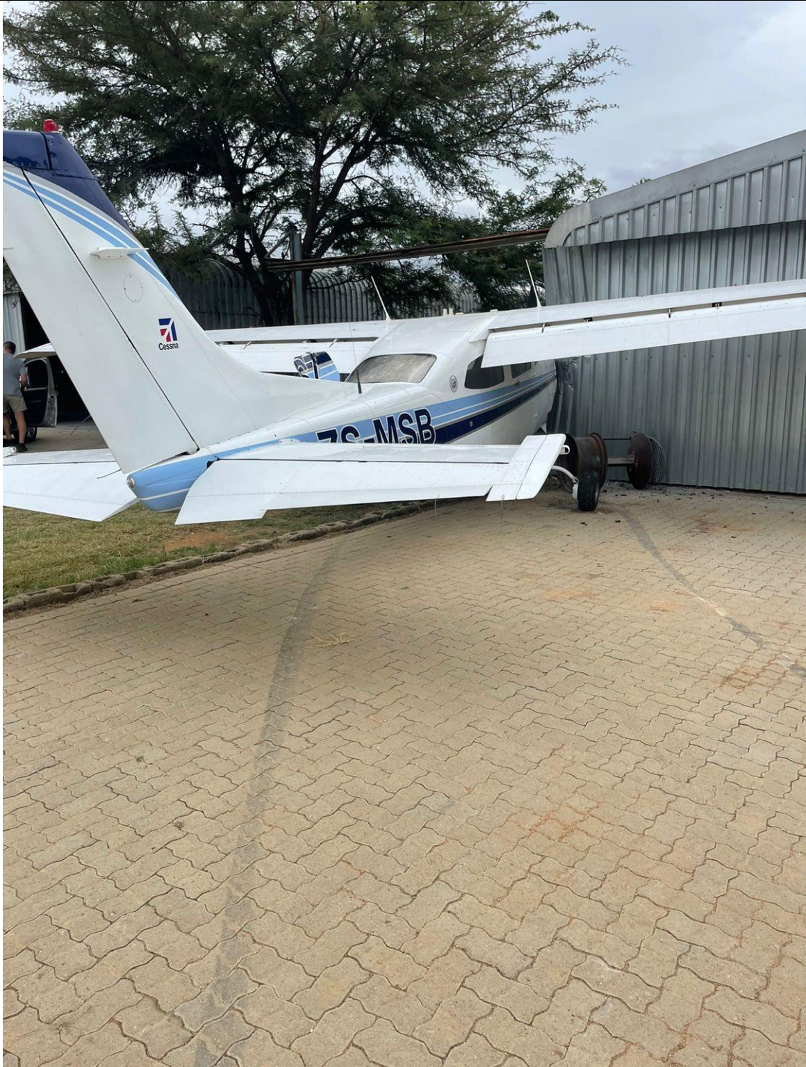
Figure 3: Tyre/brake markings from the left and the right wheels following excessive braking.
