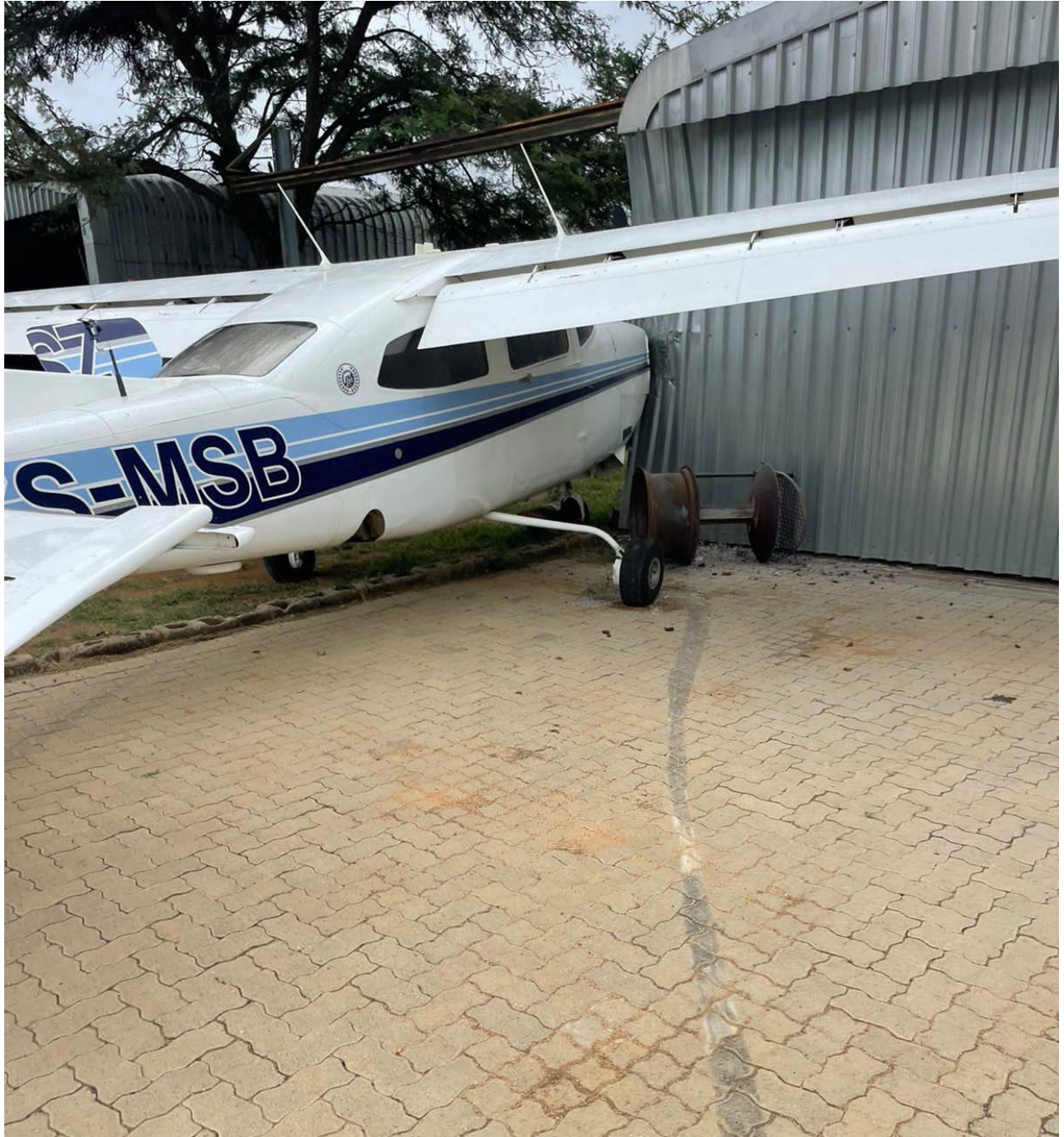
Figure 4: Tyre markings on the paving from the right wheel whilst brakes were applied.
