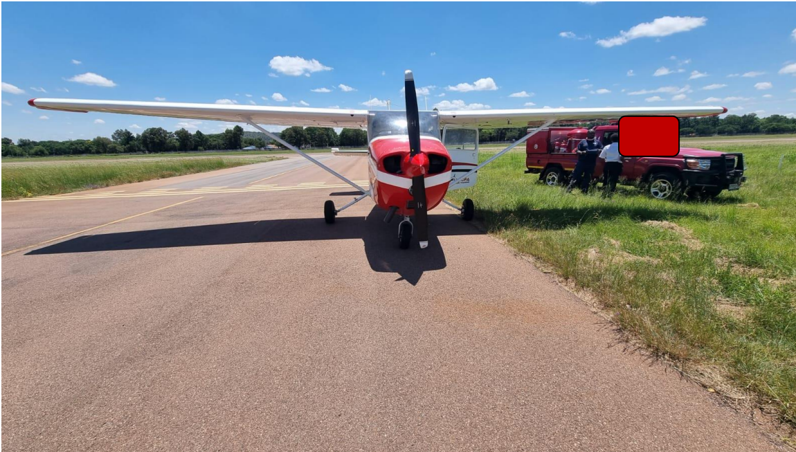
Figure 1: The damaged propeller tips and the bent nose undercarriage. (Source: Operator)
