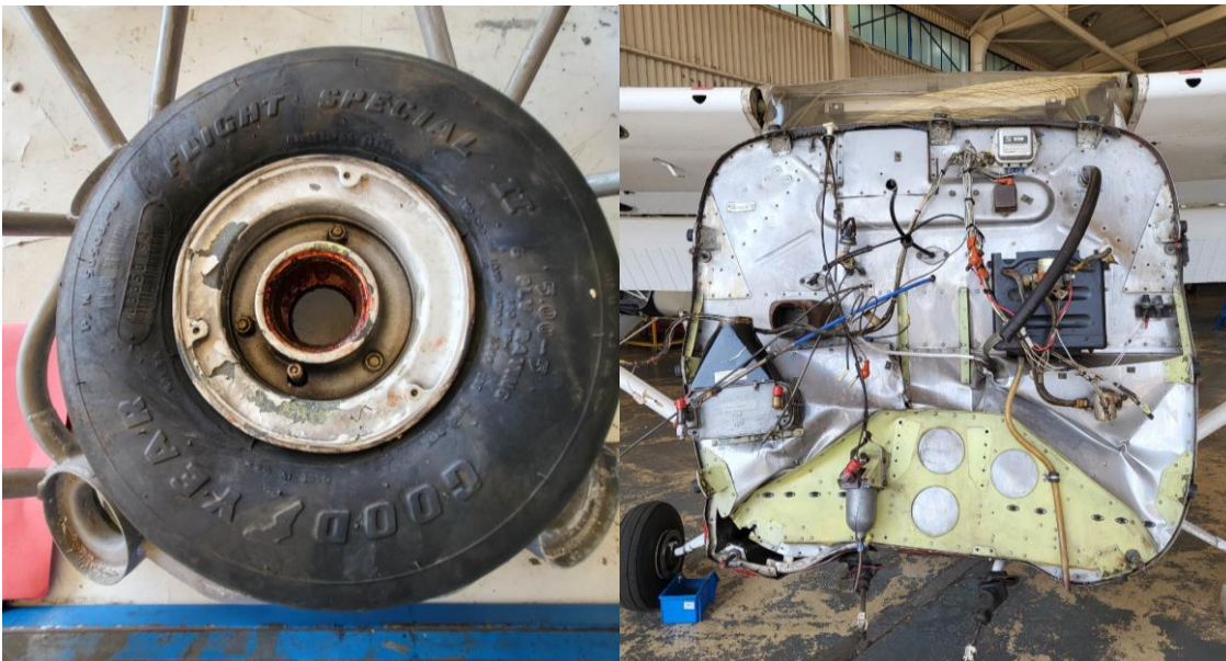
Figure 2: Damage to the nose wheel hub and the firewall.
