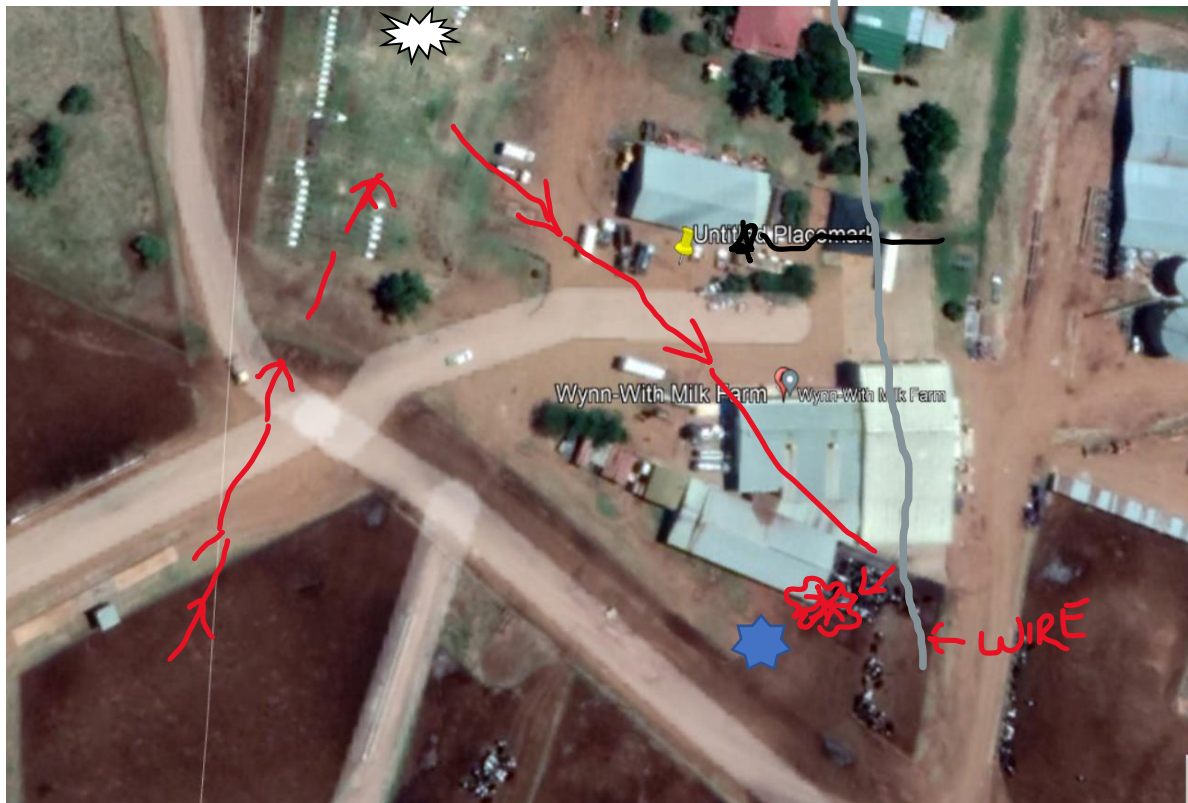
Figure 1: The white spot indicates the helicopter's first attempted landing spot. The blue spot indicates the crash site. (Source: Google Earth)
