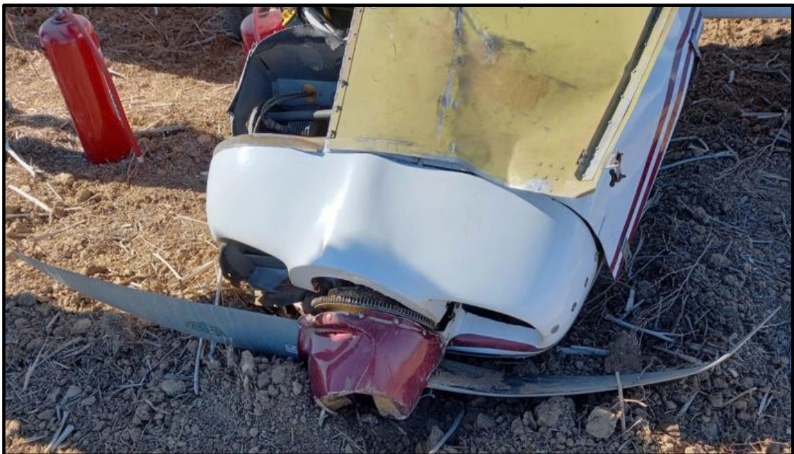
Figure 5: The damaged propeller hub and propeller blades.
