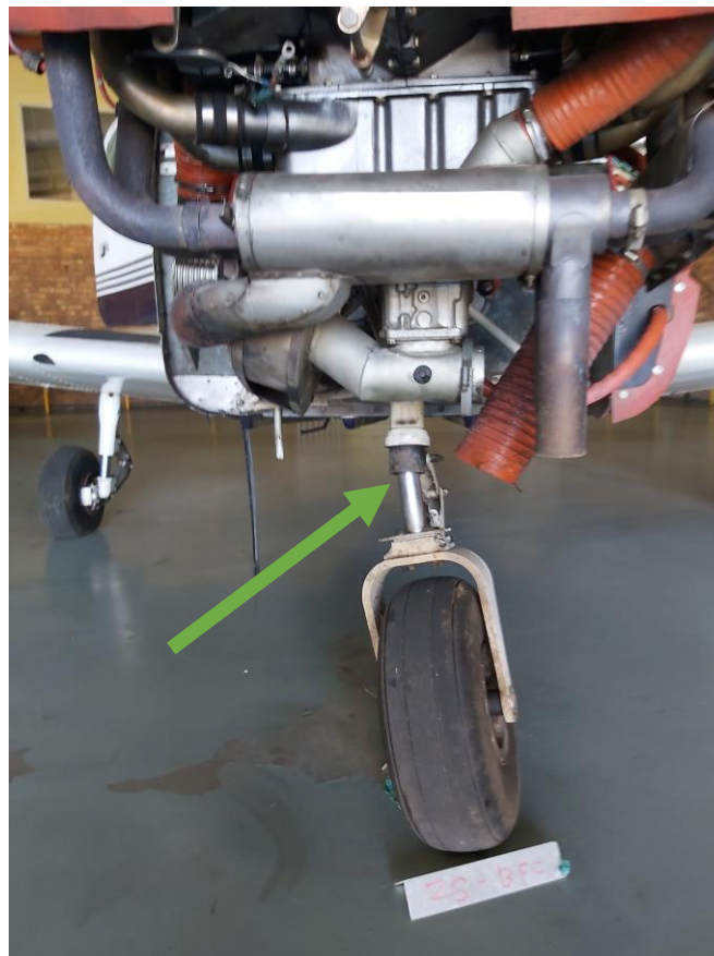
Figure 5: Arrow showing the bent nose landing gear shock absorber.
