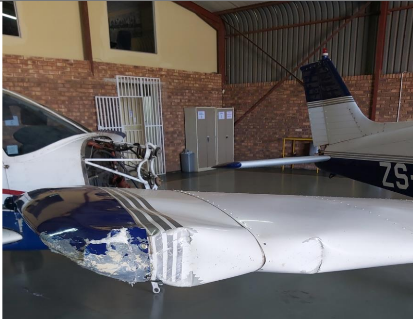
Figure 4: Damage to the right wing leading edge outboard.
