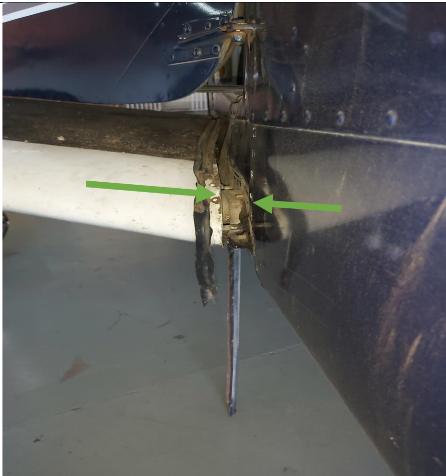
Figure 3: Arrows showing separation of the right-side wing from the fuselage.
