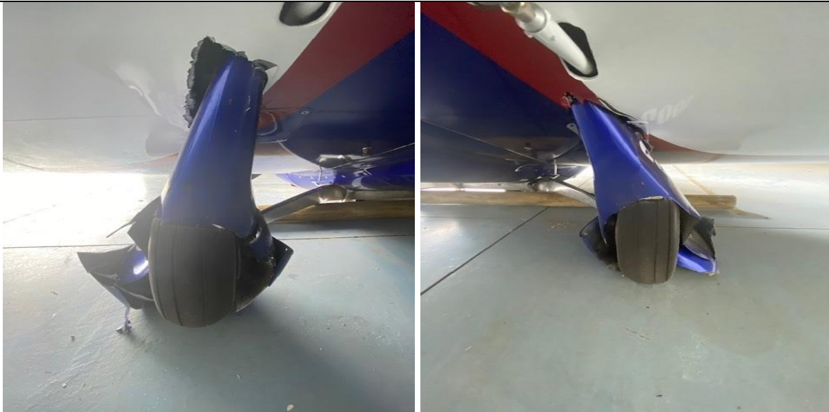
Figures 9 and 10: The left and right main landing gear struts showing the wheel fairings that cut through the underwing structure.
