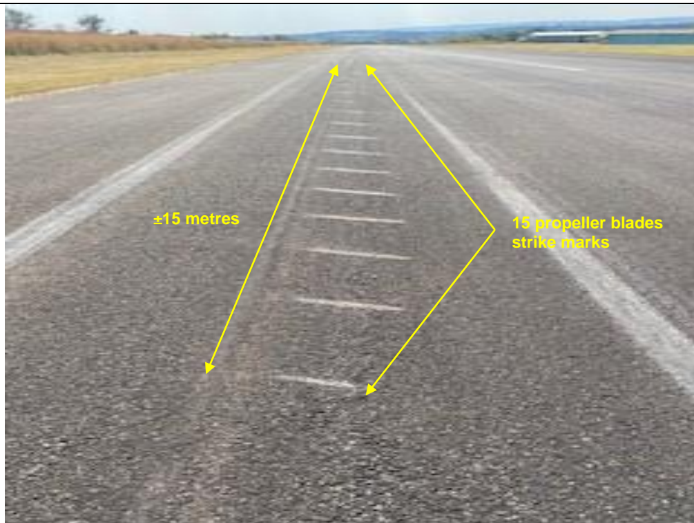
Figure 2: Propeller blades strike marks on the runway.
