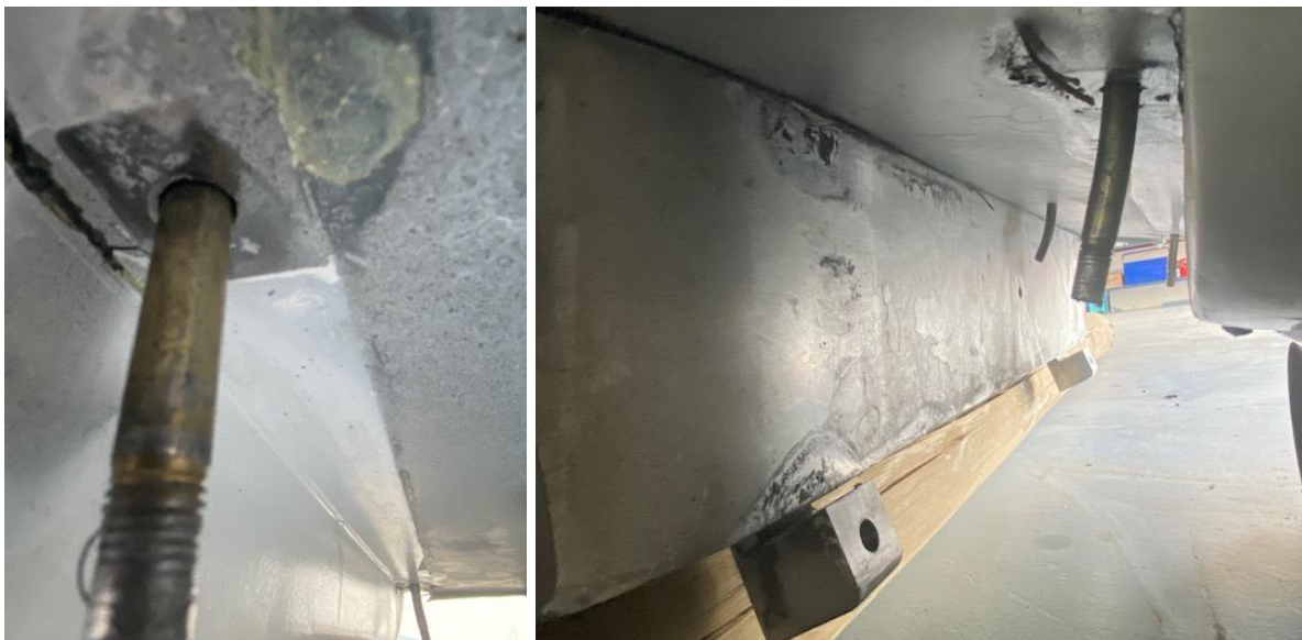
Figures 7 and 8: Stripped threads on the landing gear's left front bolt (left picture). Stripped threads on the landing gear's front right bolt (right picture).
