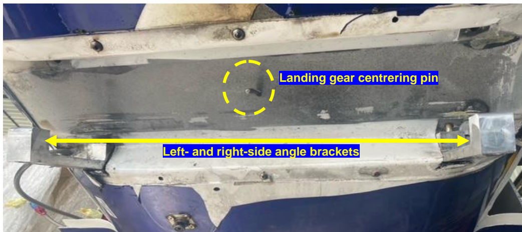
Figure 3: The saddle brackets holding the landing gear to the under-fuselage.
