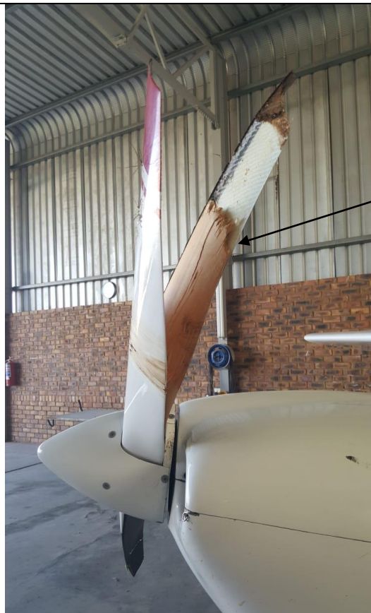
Figure 3: Damaged propeller blades. (Source: Pilot)
