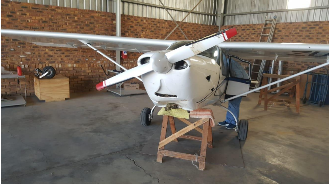
Figure 1: The aircraft without the nose gear strut after it was recovered. (Source: Pilot)
