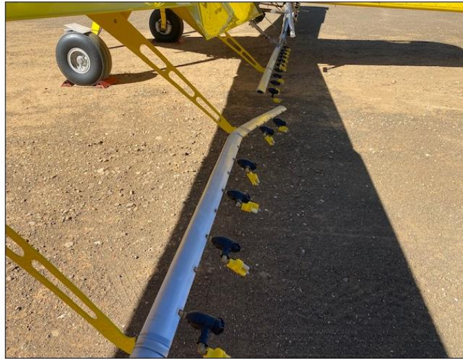
Figure 3: The broken left-side spray boom and damaged boomhangers. (Source: Pilot)
