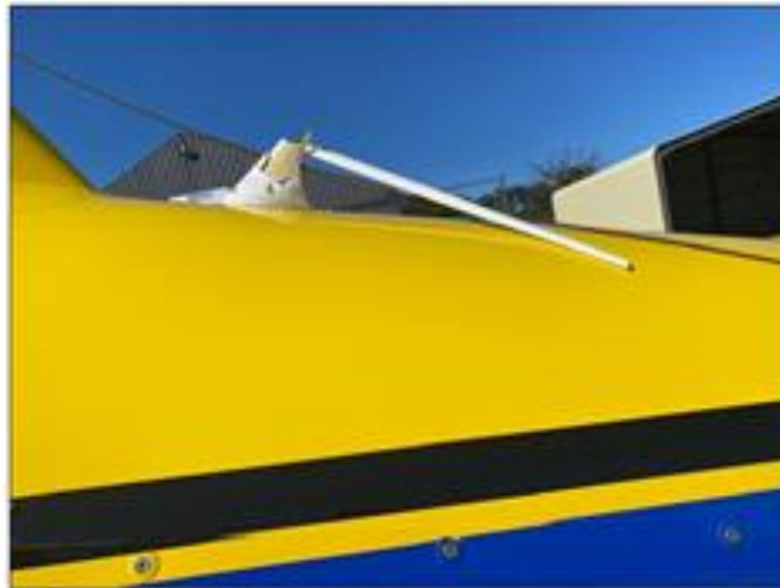
Figure 4: The broken emergency locator transmitter (ELT) and very high frequency (VHF) communication antennae. (Source: Pilot)
