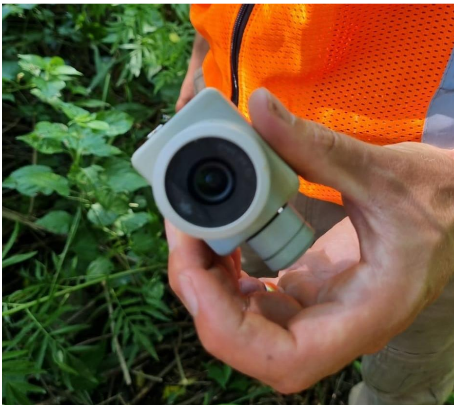
Figure 2: The gimbal that broke off. (Source: Pilot)
