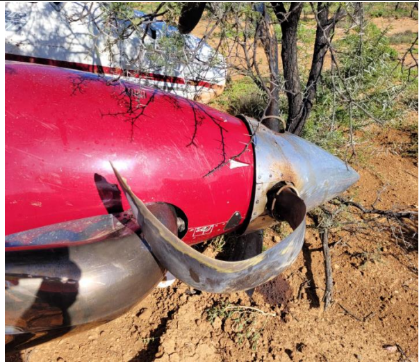
Figures 3 and 4: Left- and right-side propeller damages.
