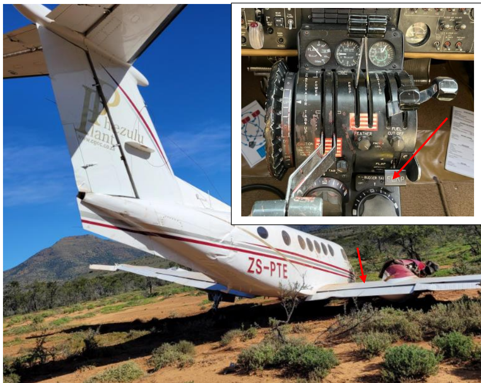
Figure 5: Flap position (take-off/approach position) viewed from the rear. The inset picture indicates flap lever position and the master switch in the 'off' position.
