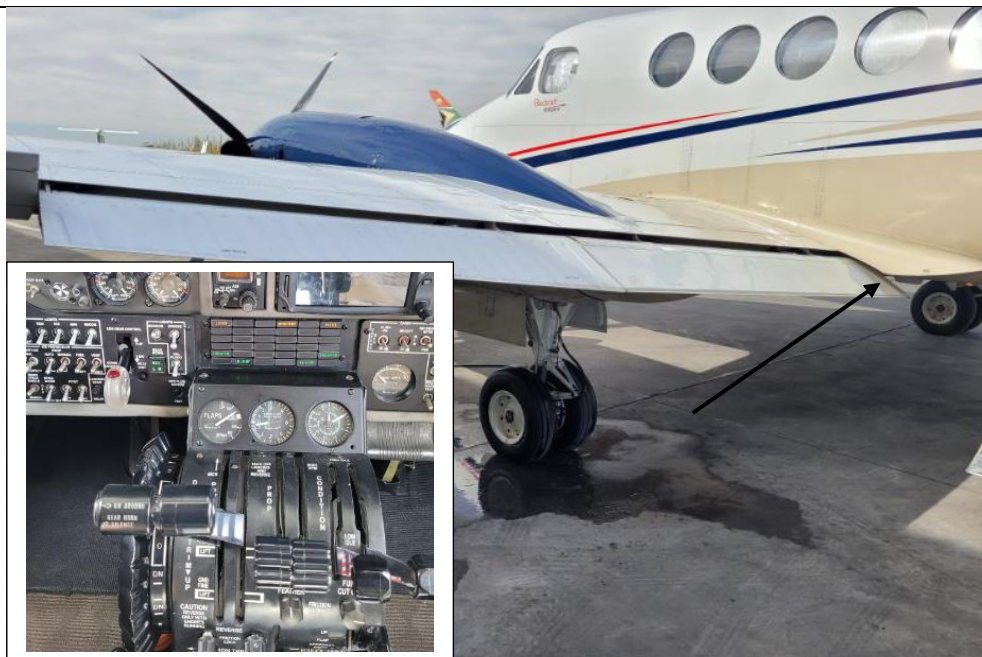
Figure 6: Flap position (take-off/approach position) comparison on a serviceable aircraft. The inset picture shows flap position and the master switch in the 'on' position.
