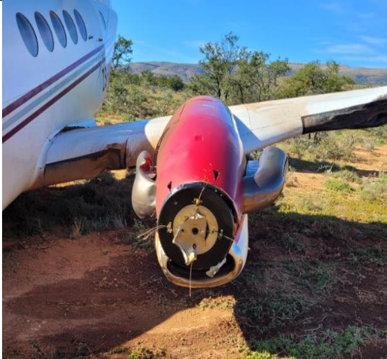
Figures 3 and 4: Left- and right-side propeller damages.
