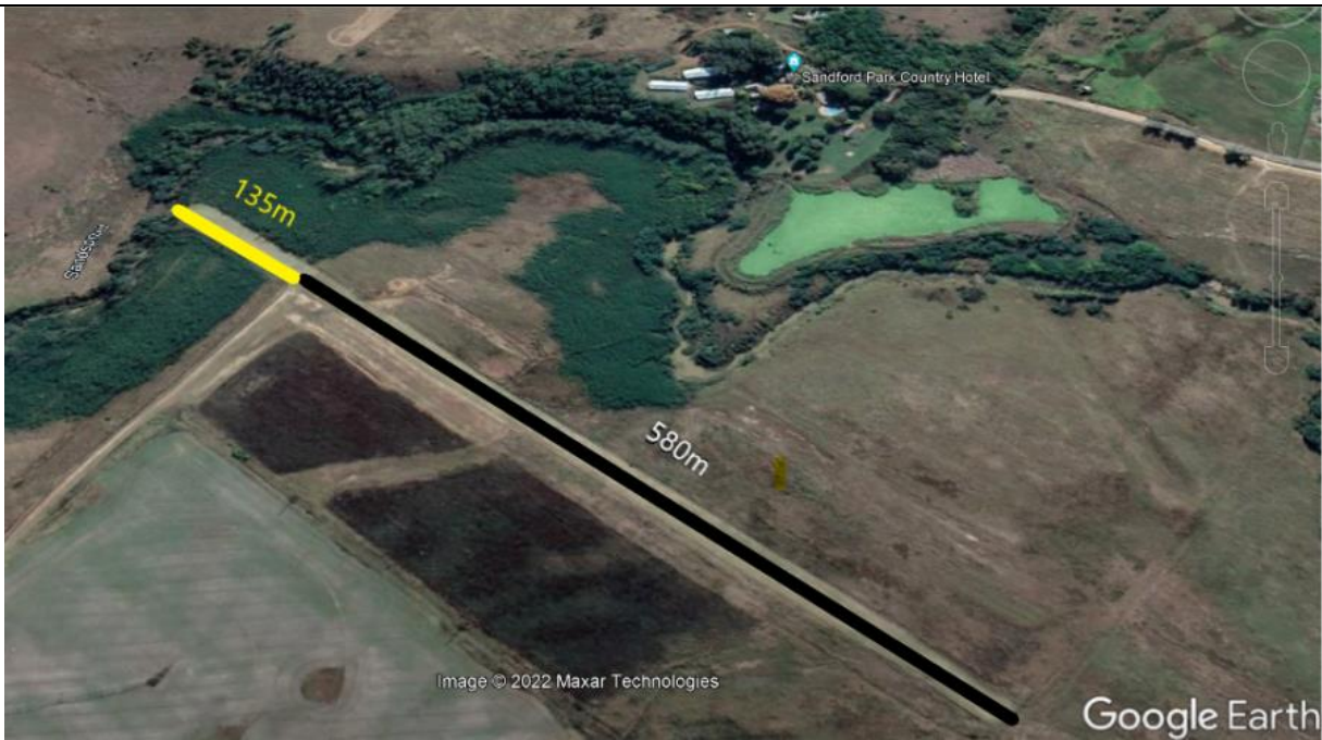
Figure 2: The runway length was adequate as for the aircraft could stop in 410ft (128m). (Source: Google Earth)
