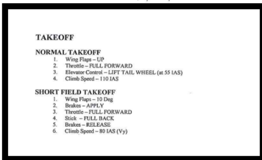
Figure 1: The short field take-off configuration to clear a 50-foot obstacle. (Source: Owner)
