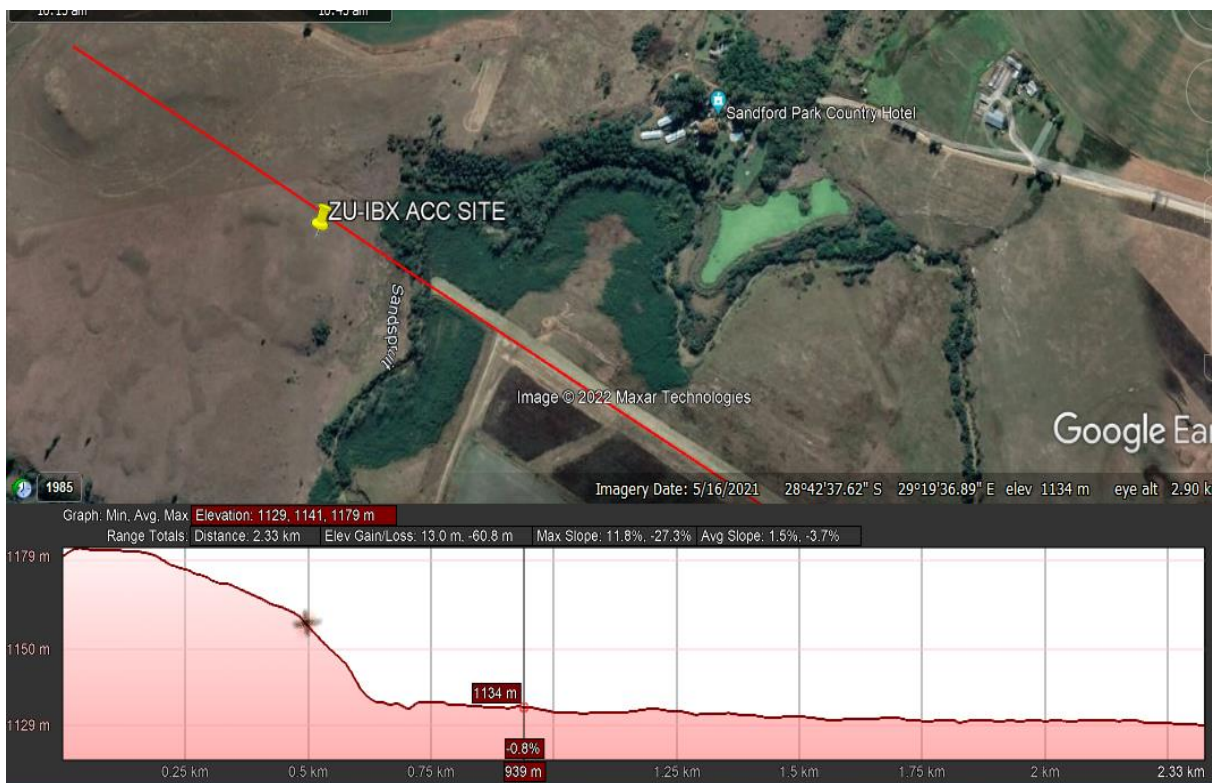
Figure 3: The aircraft was unable to clear the inclined terrain ahead of the runway, and it impacted the terrain at 67.2 feet above ground level. (Source Google Earth)
