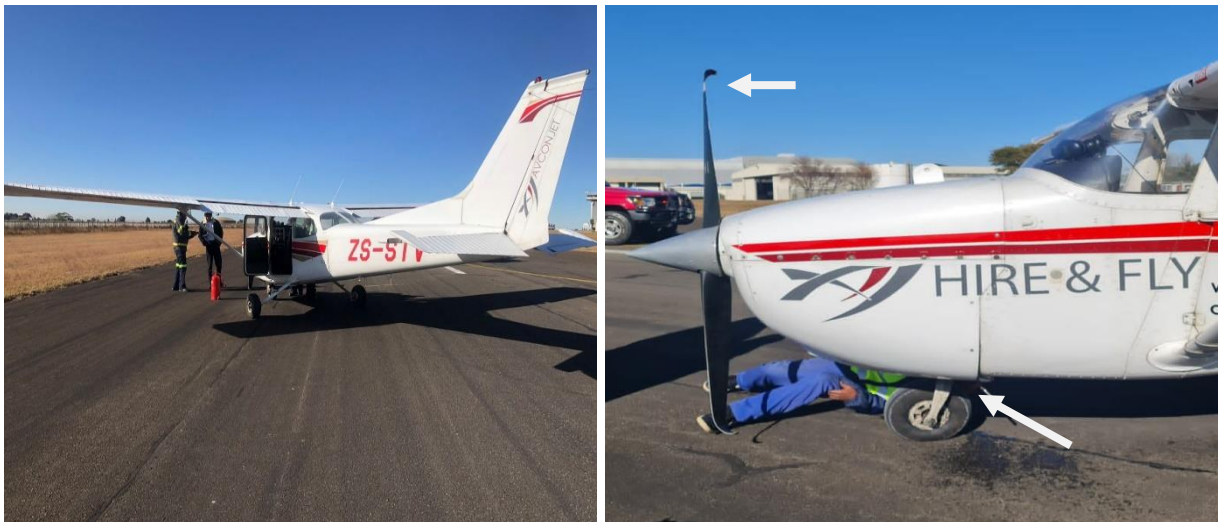
Figures 1 and 2: The aircraft on the runway (left picture). The aircraft with the arrow shows the bent propeller blade tips and nose gear (right picture). (Source: Operator)
