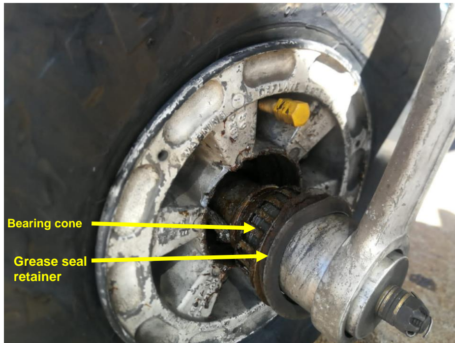
Figure 3: The nose wheel assembly. (Source: Operator)
