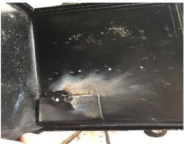
Figure 2: The damage sustained by the battery, battery lid and damaged wires
