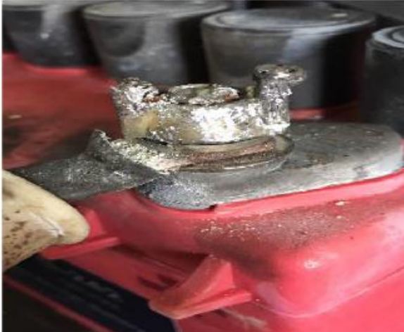
Figure 2: The damage sustained by the battery, battery lid and damaged wires
