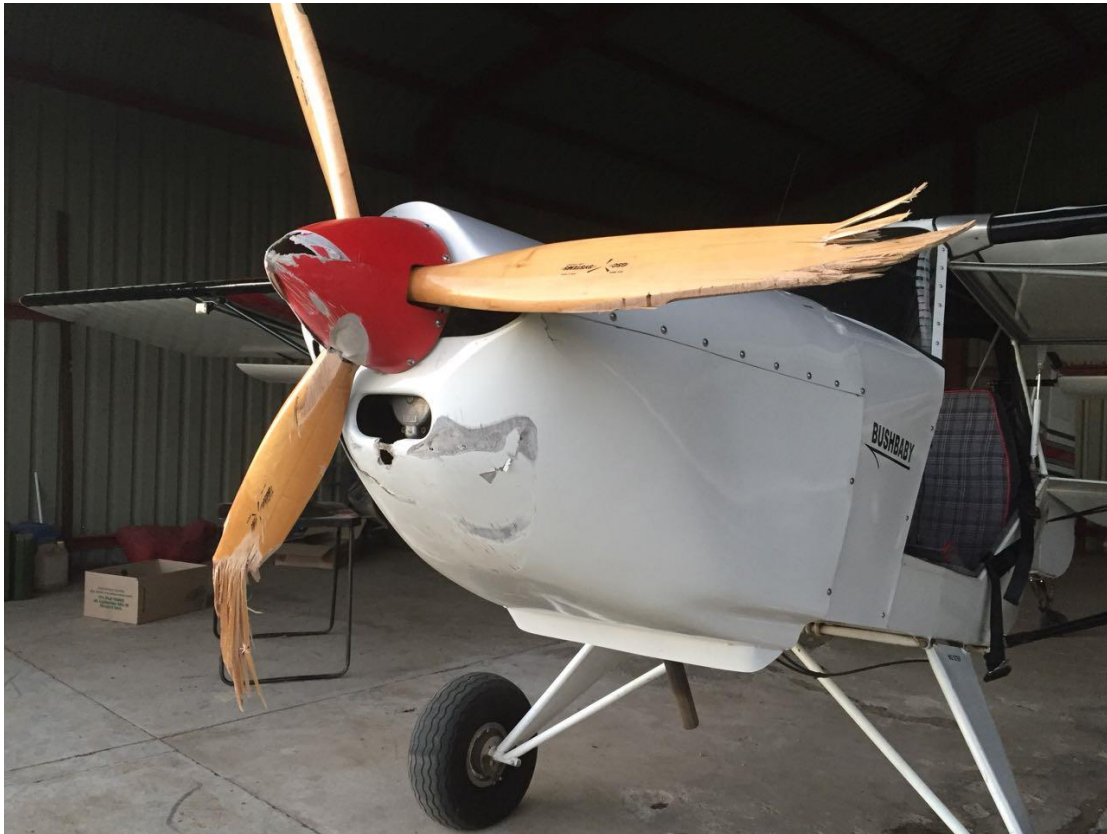
Figure 1: Damage sustained to the aircraft (source: L le Roux)
