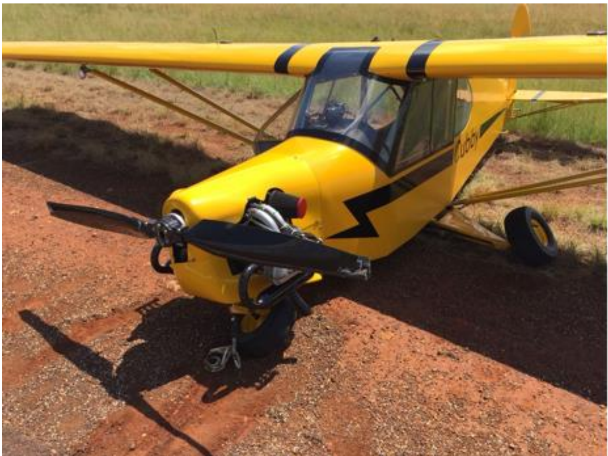
Figure 3: Damage to the landing gear and propeller (photograph courtesy of Mr J Bronkhorst)
