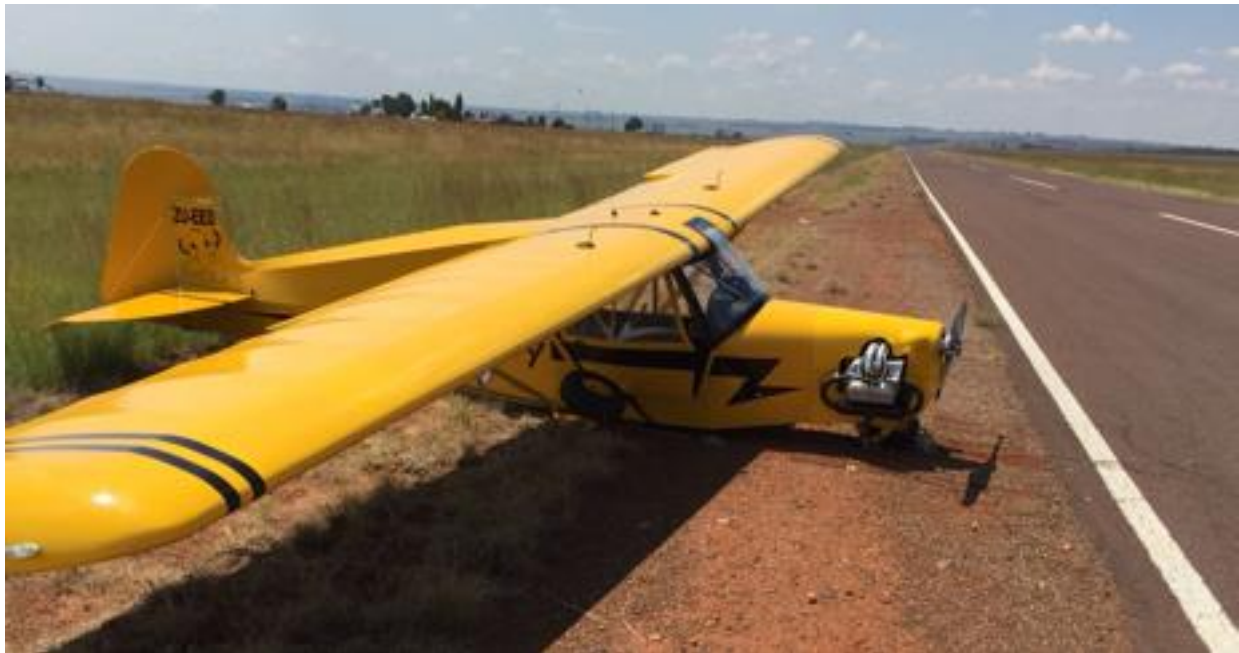
Figure 2: Damage to the landing gear (photograph courtesy of Mr J Bronkhorst)
