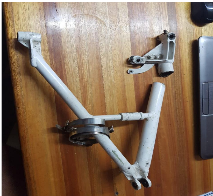
Figure 3: Broken brace assembly
