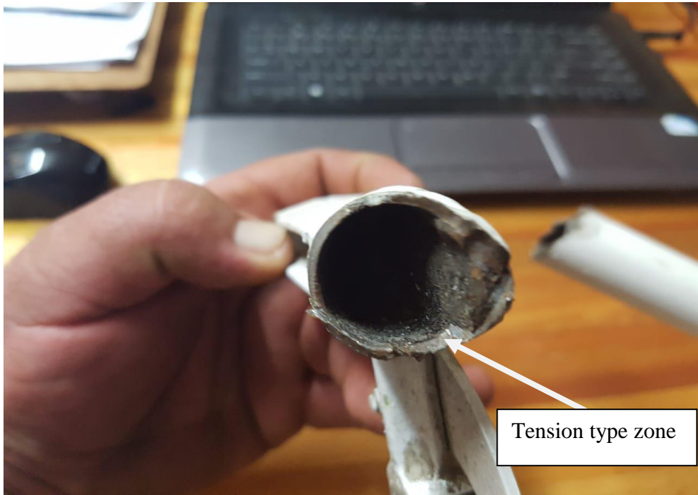
Figure 4: Shows damage to the metal
