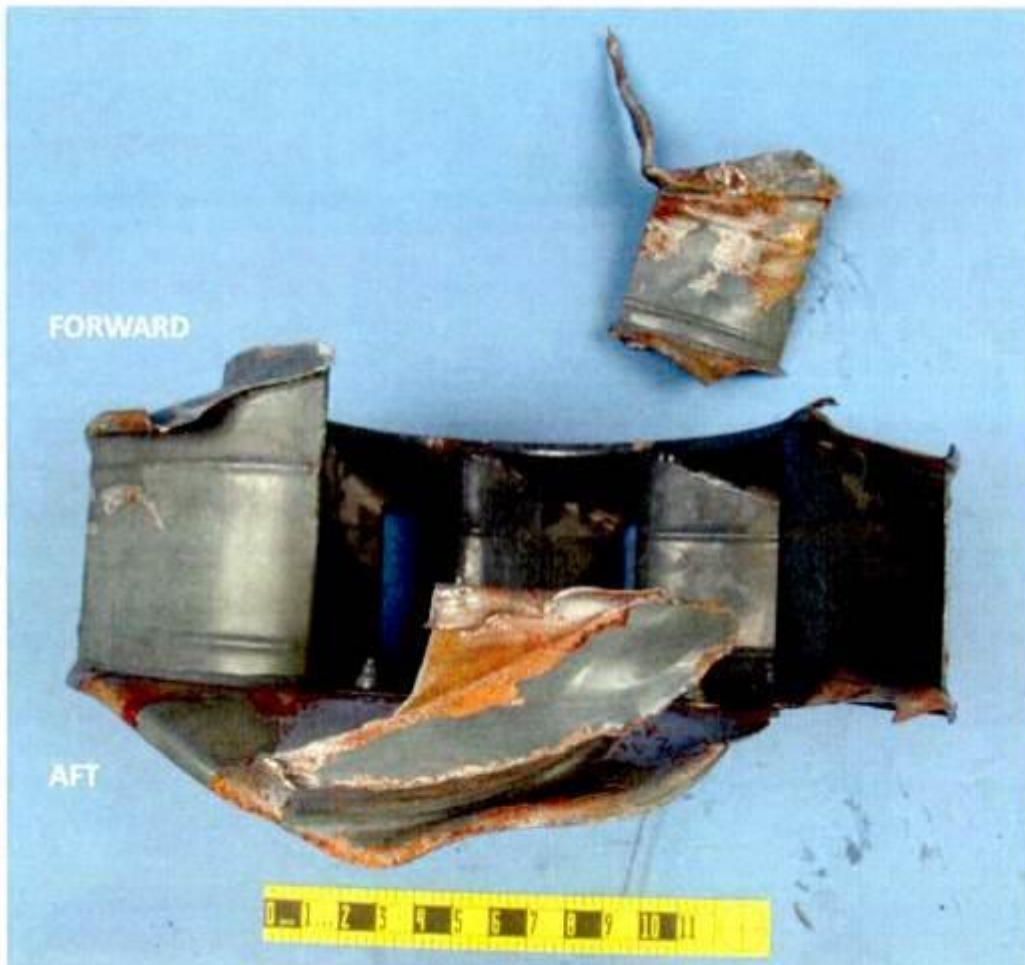
Figure 2: Overall photo of the separated cooling fan as viewed from the outer diameter.
