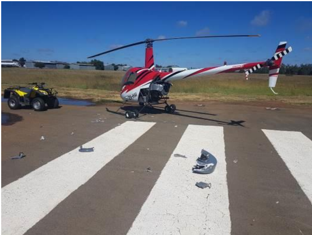
Figure 1: Debris from the fan-wheel assembly and the scroll scattered on the apron area
