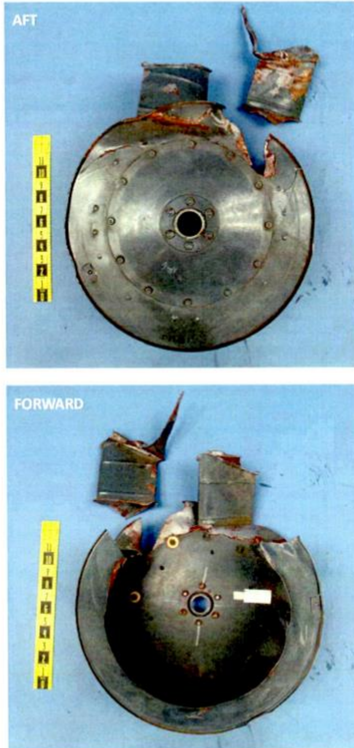
Figure 1: Overall photos of the separated cooling fan as viewed from the aft (top) and forward (bottom) sides.
