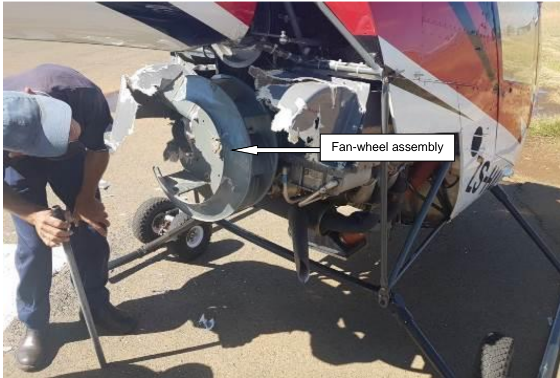
Figure 2: A closer view of the failed fan-wheel assembly
