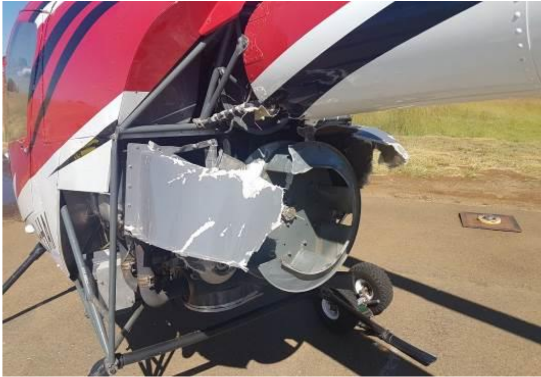
Figure 3: Another view of the damage caused by the fan-wheel assembly
