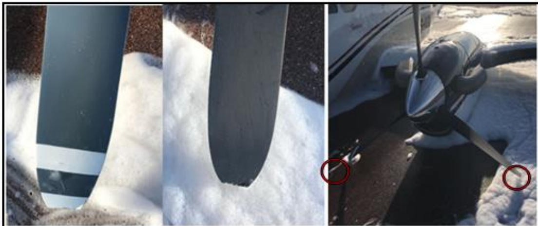
Figure 7: Damage to four propeller blades; two on each engine side
