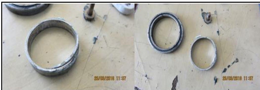
Figure 13: The damaged sleeve as it was found
