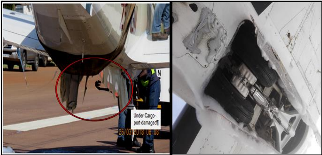
Figure 6: Damage on the under cargo port and the main landing gear doors
