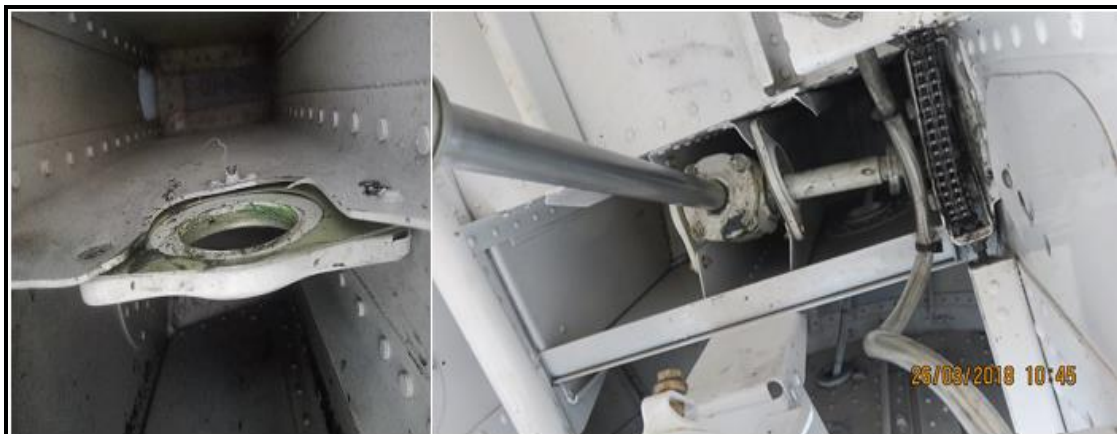
Figure 11: The actuator assembly bracket that got damaged
