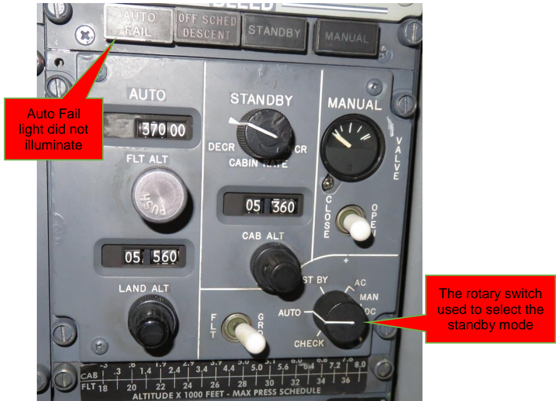
Figure 4: The aircraft pressurisation controls
