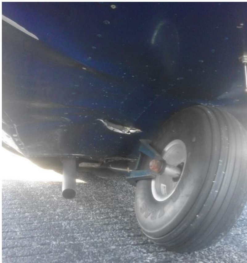
Figure 1: A view of the collapsed nose gear (source: C Coetzee)
