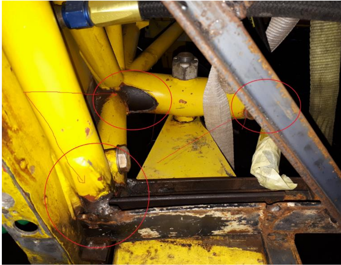
Figure 3: Damage to aircraft structure.
